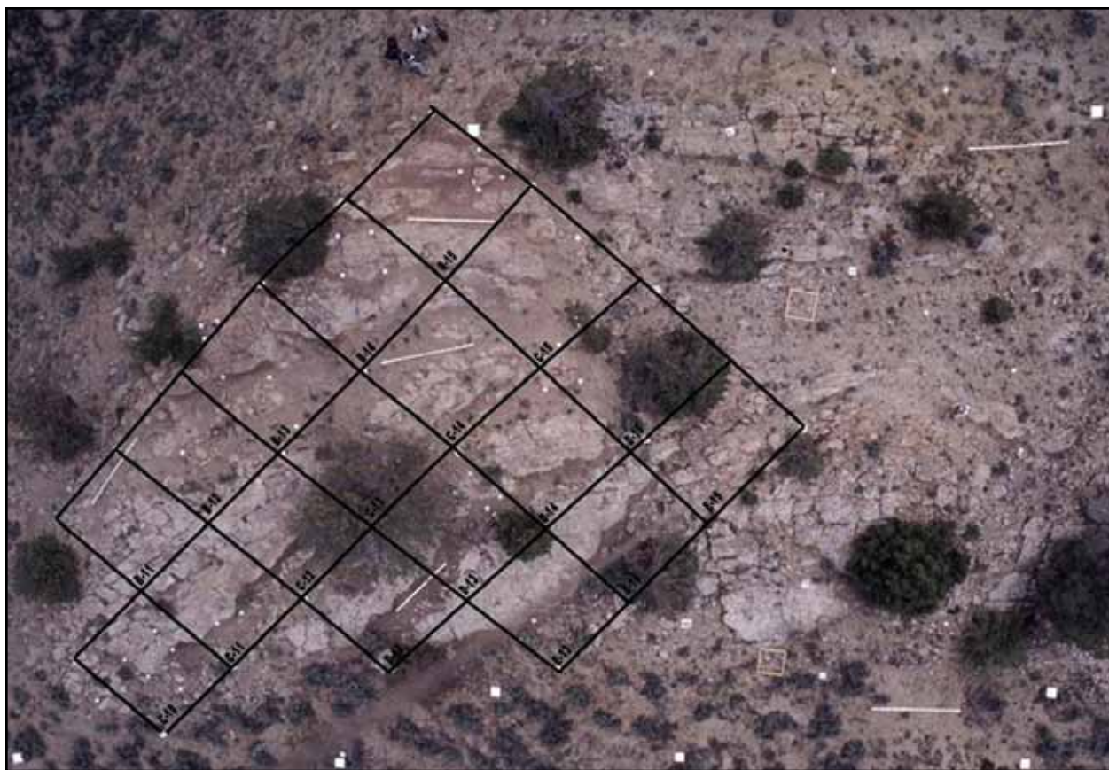
FIGURE 8. Grid created from the aerial photograph using the ACBS. Grids are 5 m (16 ft) squares. Large ornithopod track preserved as a natural cast (Fig. 12) can be seen in the upper right side of the uppermost grid (Grid B15). In addition five standard survey stadia rods and two wooden, two-meter square grids can be seen in this figure.
