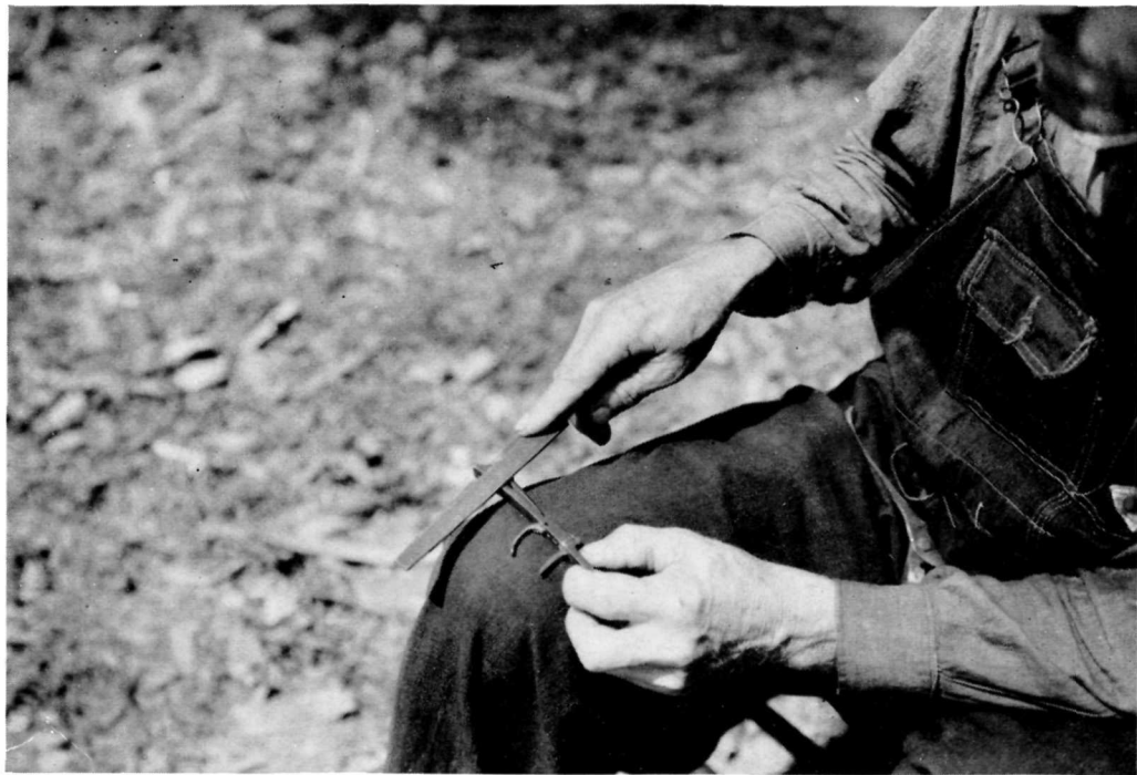
Figure 12. Details of double (set) trigger for a rifle
