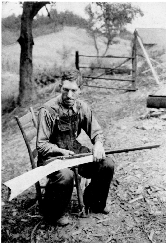
Figure 13. Making the stock for a rifle
