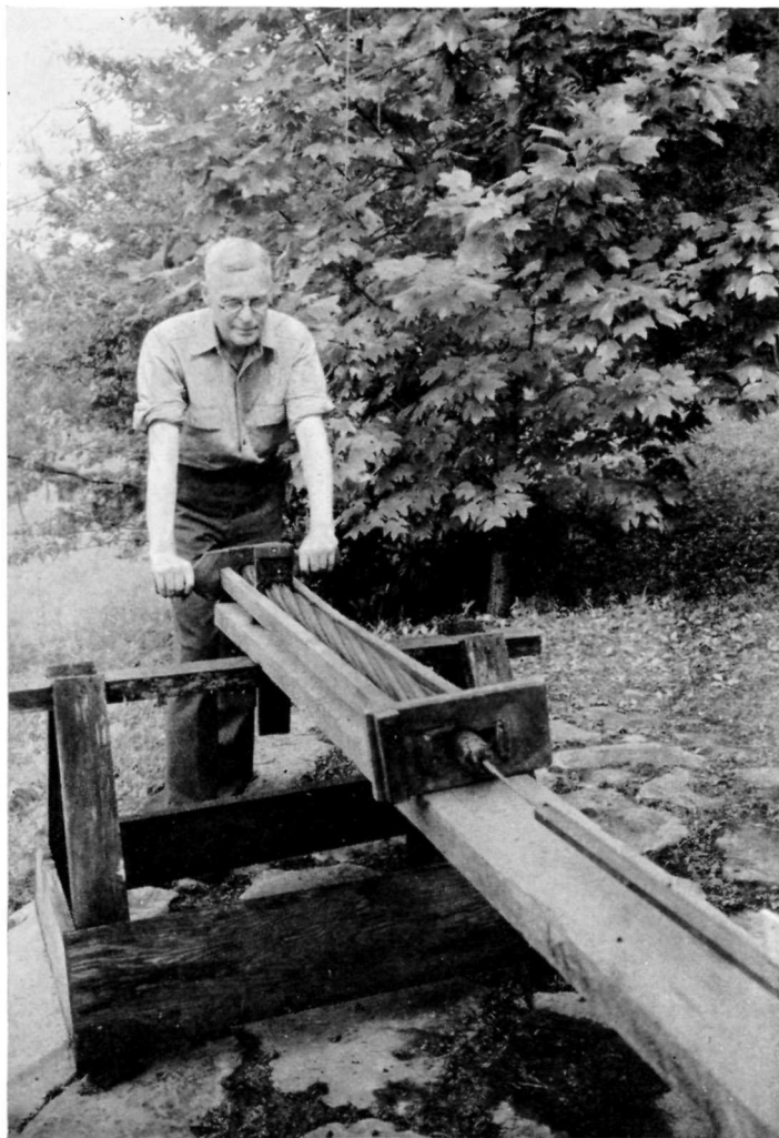
Figure 6. Rifling guide set up showing head block and part of rifling rod fastened to rifling guide and inserted into barrel of rifle
