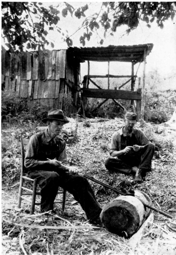
Figure 8. Dressing out the barrel of a rifle with a dressing stick
