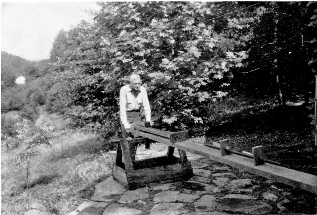
Figure 7. Complete assembly for rifling a gun—rifling guide, head block, rifling rod, and barrel of rifle
