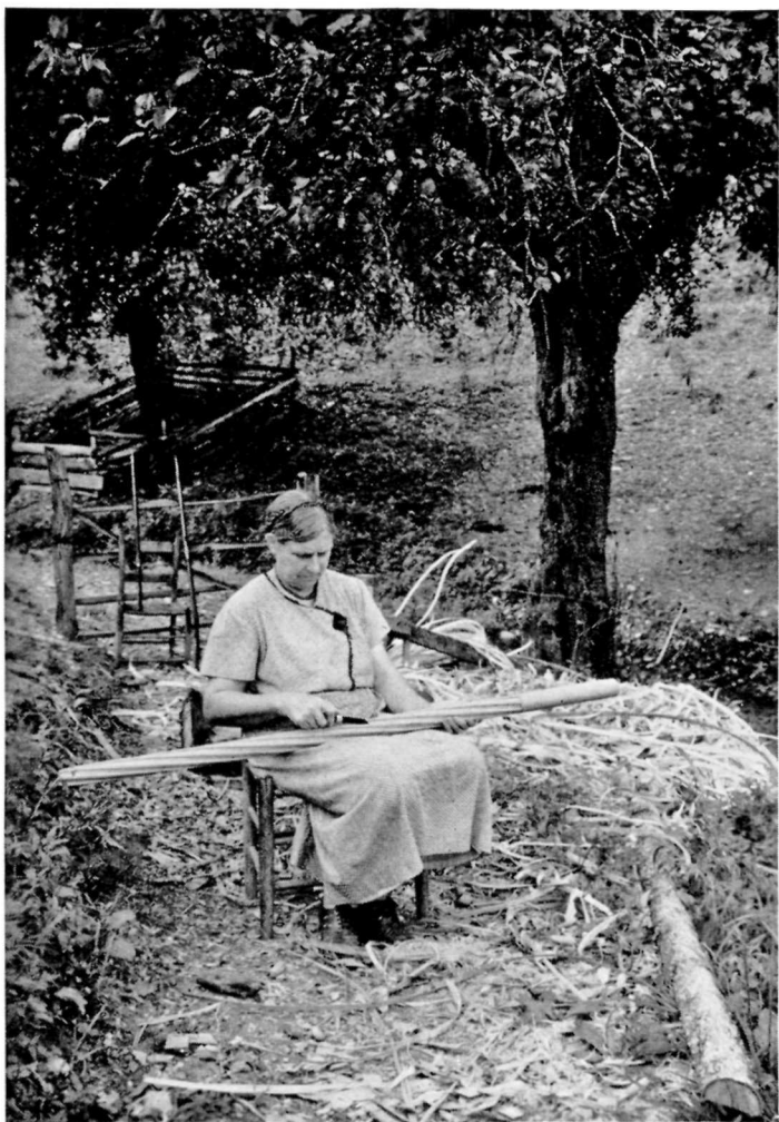
Figure 4. Cutting the rifling guide
