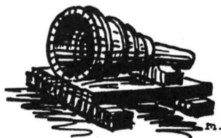
FIGURE 4—EARLY SMALL BOMBARD (1330). It was made of wrought-iron bars, bound with hoops.
