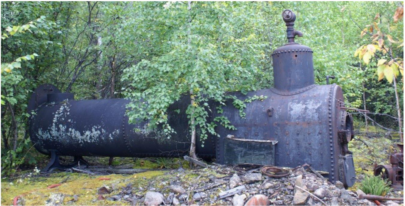
Figure 5. Photograph of a steam boiler at Coal Creek. This steam boiler is one of several obsolete mining machines that can be found in the Coal Creek Historic Mining District. The steam boiler was used by miners to thaw out sediment before sifting through it for gold. This step was necessary because the area is underlain by permafrost, meaning the ground stays frozen all year. NPS photograph by Chris Allan.
