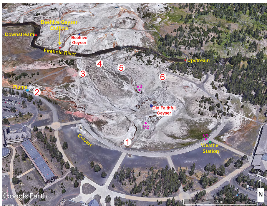
Fig. 2. Aerial image of Old Faithful Geyser and its surroundings. The red numbered labels on white backgrounds refer to outflow channels. Water flowing southward in channel number 1 is diverted by a culvert and then merges with channel number 2, which then flows towards the flume and from there to an open meadow to the northwest. Outflow channels 3–6 flow into the Firehole River. Continuous specific conductance measurements and campaign sampling of water for chemical analysis were carried out upstream and downstream from where channels 3–6 enter the river. Continuous specific conductance measurements and samples were collected on the outflow channel of Beehive Geyser before it enters the Firehole River. Also shown are the locations from which video of the eruption jet was captured (V1–V3) and the location of the weather station (V1) deployed during the experiment in April 2025. (For interpretation of the references to colour in this figure legend, the reader is referred to the web version of this article.)
