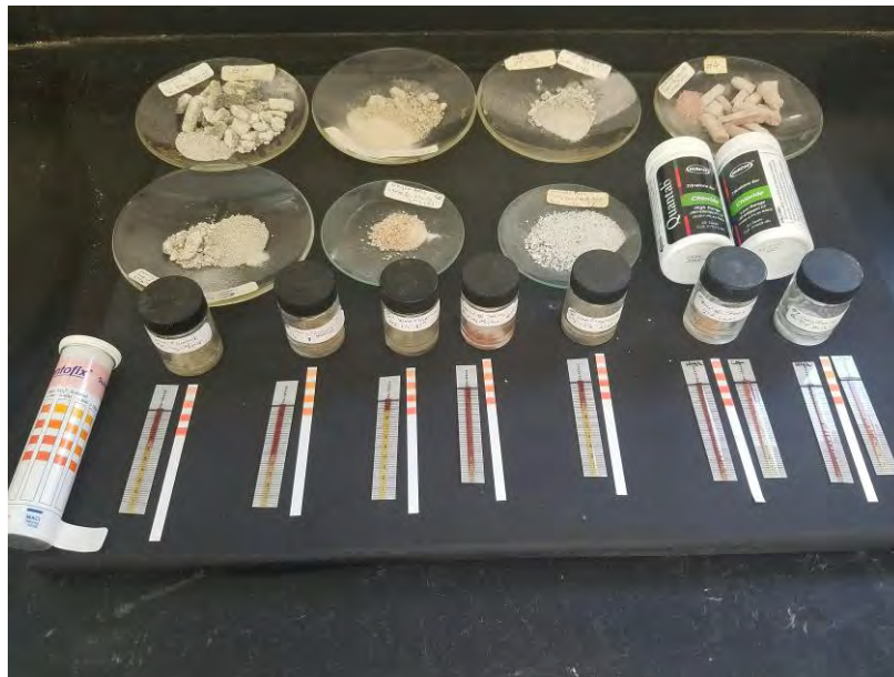
Figure 15. Mortar and stone samples tested for chlorides and sulfates.
