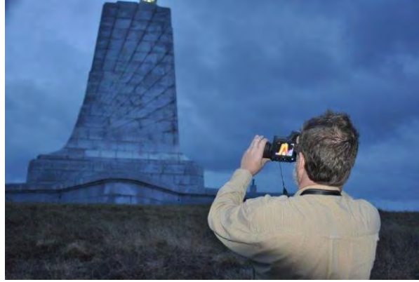
Figure 3. Infrared thermography scanning.
