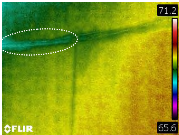
Figure 8. Interior lobby mortar joints. Water leak shows as coolness at mortar joint. Damp zones do not appear cooler indicating no evaporative cooling action.
