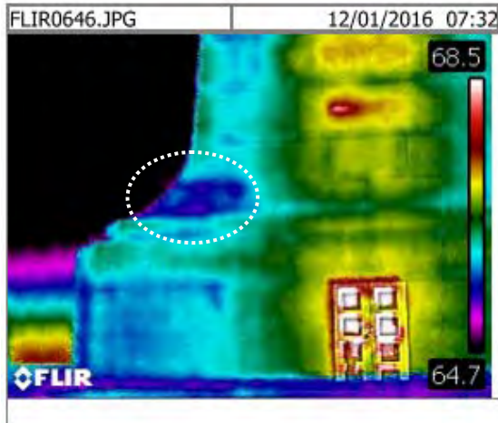
Figure 4. Exterior image taken after a rain event. Bulk water is observed and detected leaking from joints, at a joint where flashing is indicated on original construction details.
