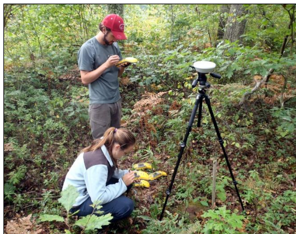
Figure 25. Promised Land State Park, PA. Ryan Hodge and Kim Oellerich test and compare accuracy of Trimble GPS units at a National Geodetic Survey marker.
