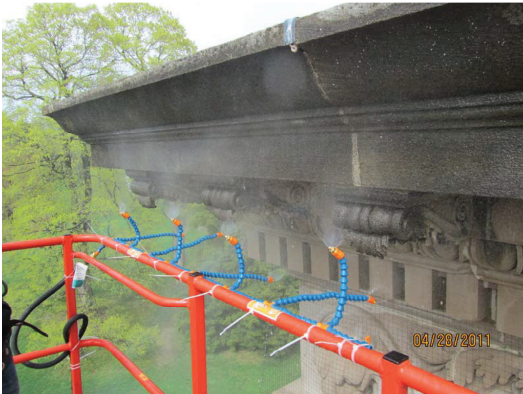
Test area #4, intermittent misting set-up
