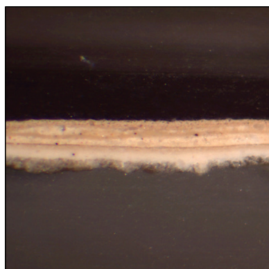
Figure 85. Photomicrographs of paint samples from the Main Stair, shown in simulated daylight on the left, and in ultraviolet light on the right. The earliest paint layer is at the bottom of each photograph. JBC, 2018.
