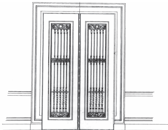
1/4" INCH SCALE DETAIL OF BRONZE GRILLE FOR VESTIBULE DOOR - HOUSE FOR F.W. VANDERBILT, ESQ. AT HYDE PARK ON THE HUDSON, N.Y. BOTH SIDES OF GRILLE TO BE THE SAME - MCKIM, MEAD AND WHITE ARCHT. 160. 5TH AVE., NEW YORK, N.Y.
