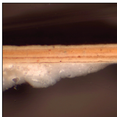
Figure 95. Photomicrographs of selected paint samples from the Servants' Hall and Pantry, shown in simulated daylight on the left, and in ultraviolet light on the right. The earliest paint layer is at the bottom of each photograph. JBC, 2018.
