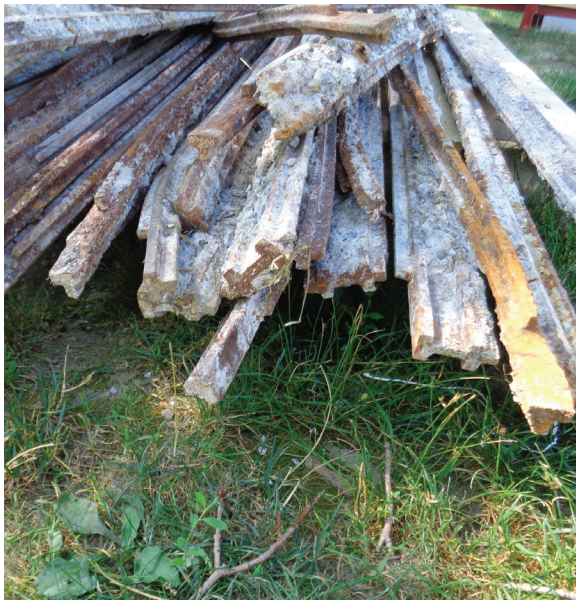
Figure 6. The mansion's framing included Columbian Fireproofing Company Reinforcing Bars. The two lower photographs show the double-T connecting bars and stirrups taken from the framing for the west porch floor. The upper drawing shows the system from the 1906 Sweets Catalog. The Architectural Record Company, "Sweet's" Indexed Catalogue of Building Construction for the Year 1906 , 105.
