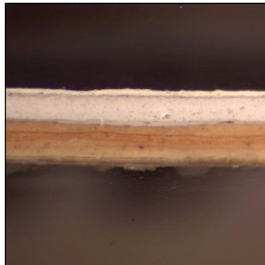
Figure 91. Photomicrographs of selected paint samples from the Butler's Room, shown in simulated daylight on the left, and in ultraviolet light on the right. The earliest paint layer is at the bottom of each photograph. JBC, 2018.
