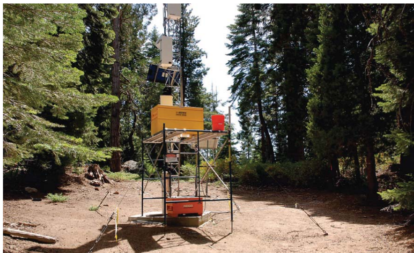
Figure 1. One of four flux towers installed at different altitudes between 405 and 2700 m by the Southern Sierra Critical Zone Observatory, California, USA. Instruments collect information about climate and fluxes of carbon dioxide and water vapor with the objective of gaining new knowledge on how water, soils, and climate interact. Photo: Claudia Drexler
