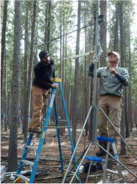
Figure 2. Scott Peckham (left) and Kevin Hyde (right) rig a sub-canopy eddy-covariance tower in Chimney Park, Snowy Mountains, Wyoming. The experiments monitor evapotranspiration response to the pine bark beetle outbreak. Photo: Elise Pendell
