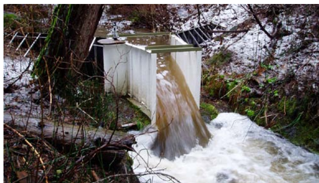
Figure 4. Fiberglass flumes provide a uniform stream cross-section for accurate stream discharge measurements. This photo shows high flow at a Providence Site stream during a rain-on-snow event that created stream turbidity (suspended sediment) which is measured at KREW. Photo: T. Whitaker
