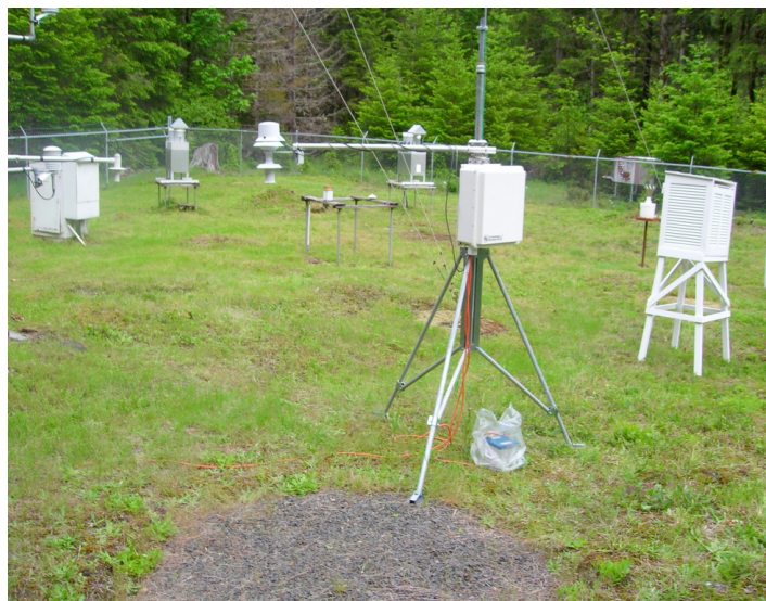
The HJ Andrews Station array of climate sensors. Photo by Melanie Lenart.
