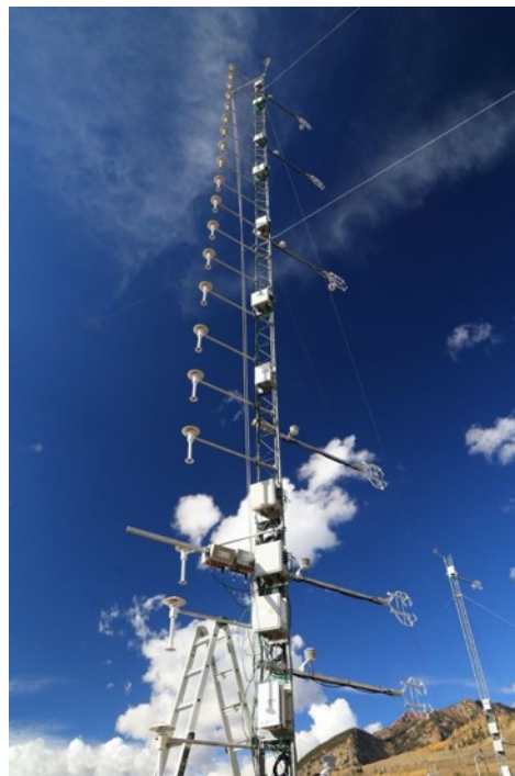
Figure 2. Looking up at the 20 m tower during October field deployment. On left, temperature and relative humidity sensors every 1 m, sonic anemometers (to measure air movement) at every 4 m. Image Credit: Emilio Mateo, AGCI.
