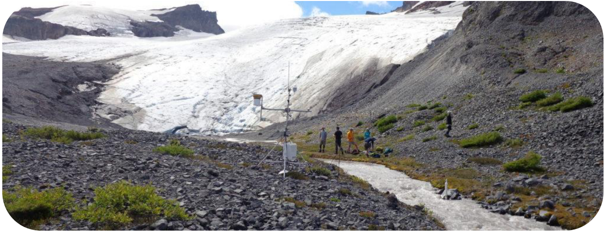
Sholes Glacier and stream gage station. We have constructed a rating curve for this station that the Nooksack Indian Tribe maintains (Grah and Beaulieu, 2013). This photo was taken below Sholes Glacier in 2015 and exhibits the darkening of the surface that occurs in high melt years, increasing melt rates. Image Credit: Jill Pelto and Mauri Pelto.
