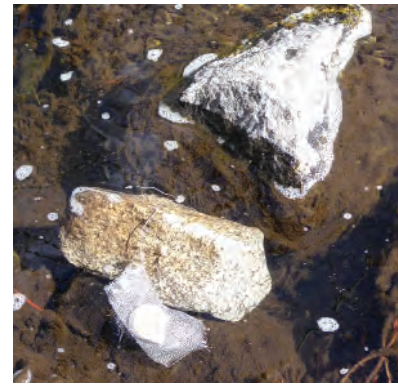
Figure 6. Use the wire to secure the package in wet places. In a) I've tethered it to a tree near snow (=wet). Here the case is unprotected from direct sunlight, but they should always be in a shaded location or in a radiation shield of some kind. In b) I'm showing the case in a stream, but again it should be protected from direct sunlight (e.g., under a rock).
