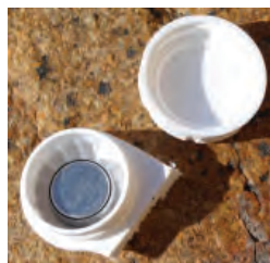
Figure 4. Here I put my programmed iButton in its new water-tight container.
