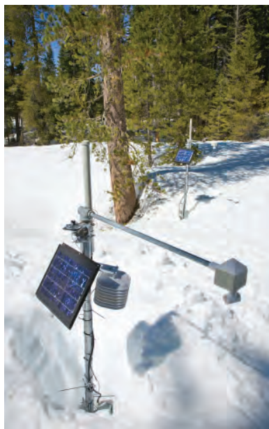
Figure 2. A strategically-placed network of solar-powered monitors capture variations in snow depth, soil moisture and temperature, air temperature and relative humidity, and solar radiation across the forest landscape every 15 minutes at Providence Creek Catchments site P301, Sierra National Forest, CA USA. Wireless-sensor networks based on these instrument clusters developed at the Southern Sierra Critical Zone Observatory have been deployed in multiple watershed headwaters in the state. Photo: Roger Wyan
