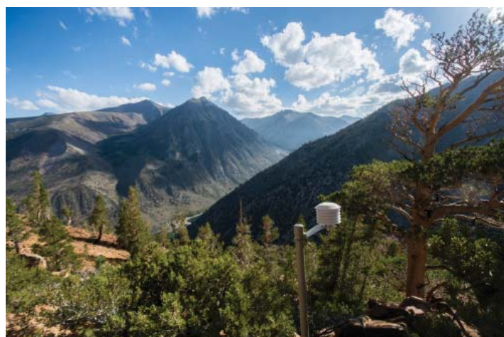
Figure 3. Sensor deployment for this study involved placing temperature loggers on elevated, open woodland slopes. Gill-type radiation shields were used to replicate temperature observations across common source data networks for PRISM.
