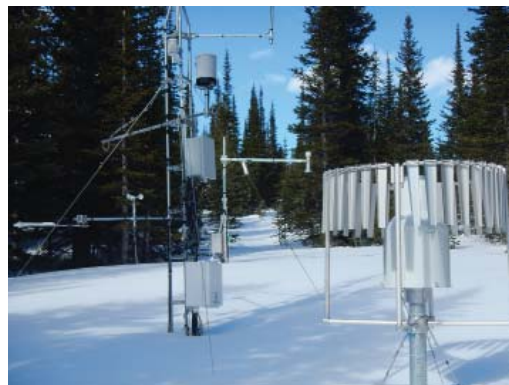
Figure 2. Powerline site at Fortress Mountain, including met tower, Pluvio, SPA, snow scale (buried) and Parsivel (not visible).
