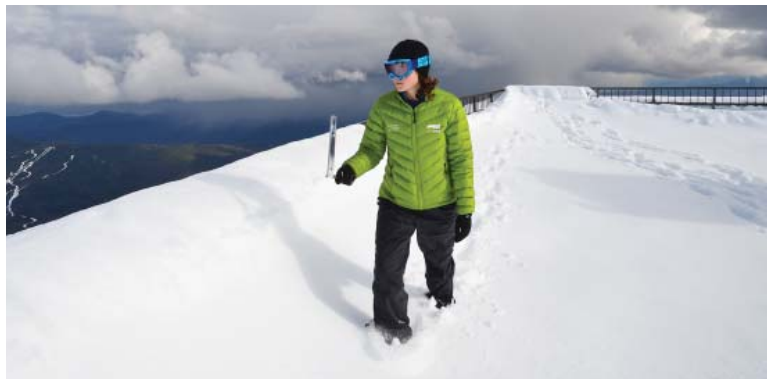
Deck Slinging: Observer Rebecca Scholand performs the hourly ritual of using a sling psychrometer to measure temperature and humidity atop Mount Washington, New Hampshire. Hourly temperature and humidity have been measured using this same method since 1932.
