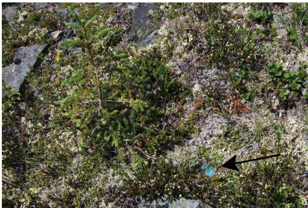
Figure 2. Sensor near treeline. Surface temperature sensors allow estimation of snowpack duration. Paired with air temperature, soil temperature, and other measurements deployed in a network, variation in watershed responses can be measured.
