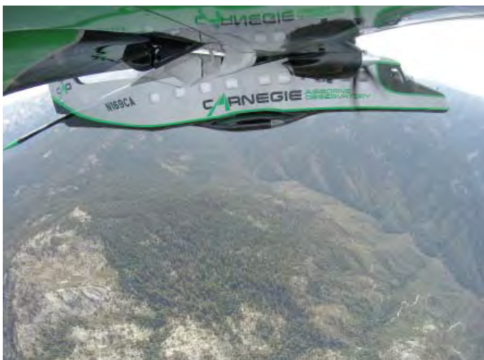
Figure 6. An aircraft captures high-resolution LiDAR and hyperspectral images of forests during the drought. Photo: G. Asner, Carnegie Institute of Science.
