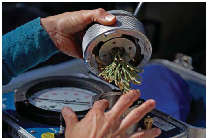
Figure 4. A pressure chamber is used to record how much pressure is required to squeeze water out of a small sequoia branch – a measure of the drought stress experienced by the sequoia. Photo: A. Ambrose, UC Berkeley.
