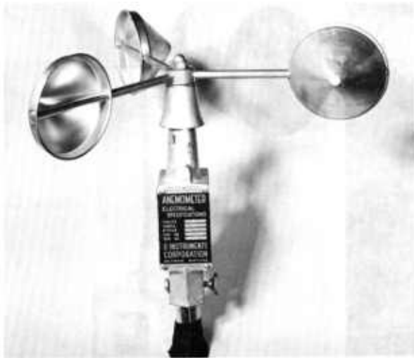
Figure 3.2. — The small Airways anemometer with 1/60-mile contacts is used at many fire-weather stations.
