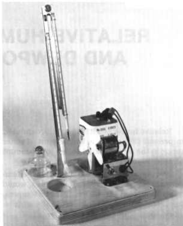
Figure 2.1. — Electric fan psychrometer, USDA Forest Service type. This instrument is recommended for use at all permanent fire-weather stations.
