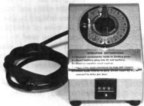
Figure 3.4. — Reset type mechanical counter with timer simplifies determination of 10-minute average windspeed.
