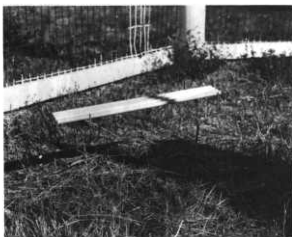
Figure 15.4. — Replace stick on wire rack, hook north, brads down.
