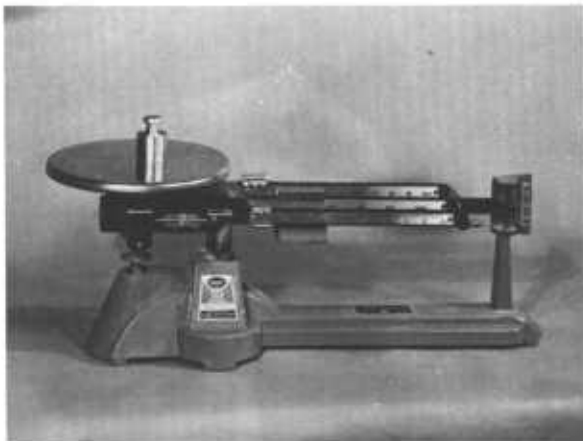
Figure 15.8. — Checking the balance of triple beam balance.
