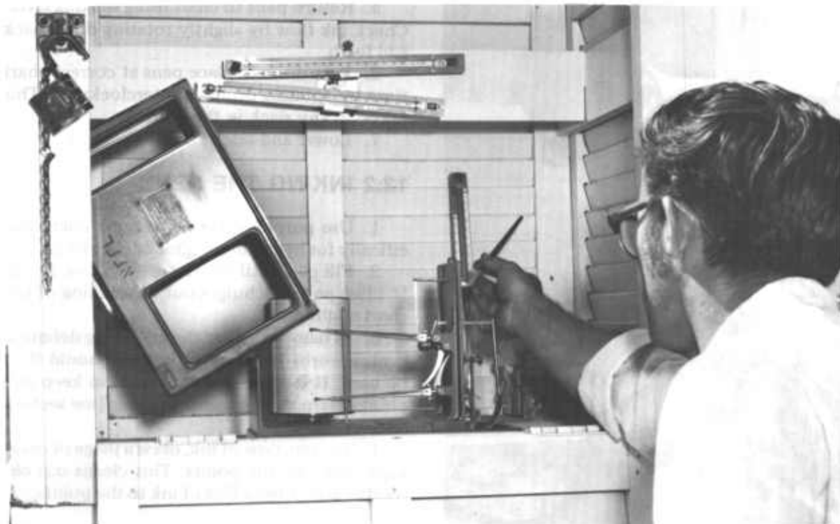
Figure 12.4. — Use a clean, dry, camel's hair brush to remove dirt and dust.
