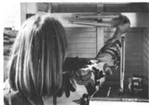
Figure 10.2. — Reading and setting maximum-minimum thermometers.
