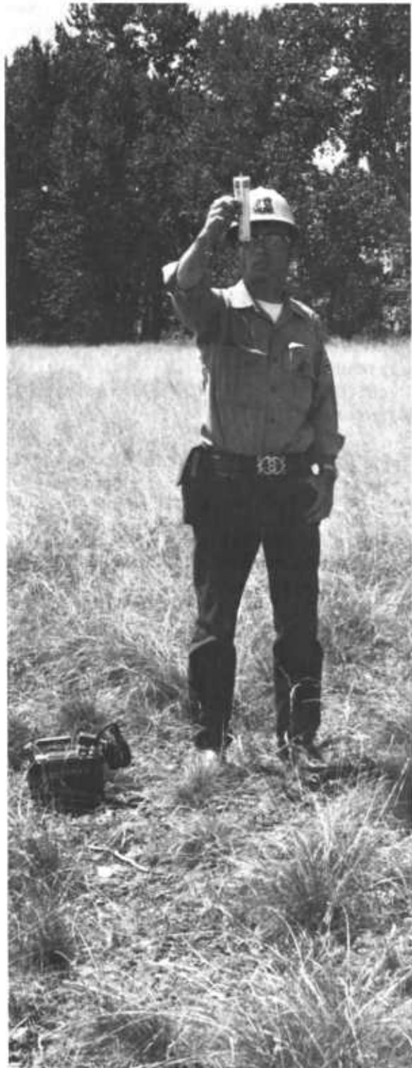
Figure 13.3. — Assume a face-into-wind position when using hand-held wind meter. Keep fingers clear of top stem when measuring winds less than 10 m.p.h.
