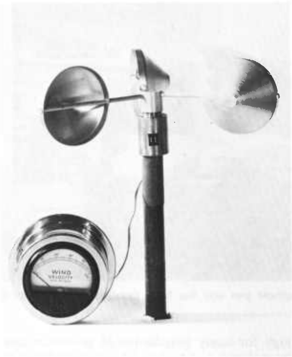
Figure 3.8. — Generator anemometer with remote dial readout is useful whenever instantaneous windspeed measurements are desired.
