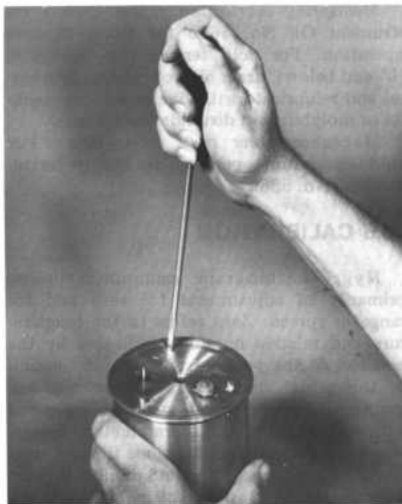
Figure 18.4. — Loosen three screws on bottom of drum and shift gear away from center of drum to correct for backlash and drag between gears.
