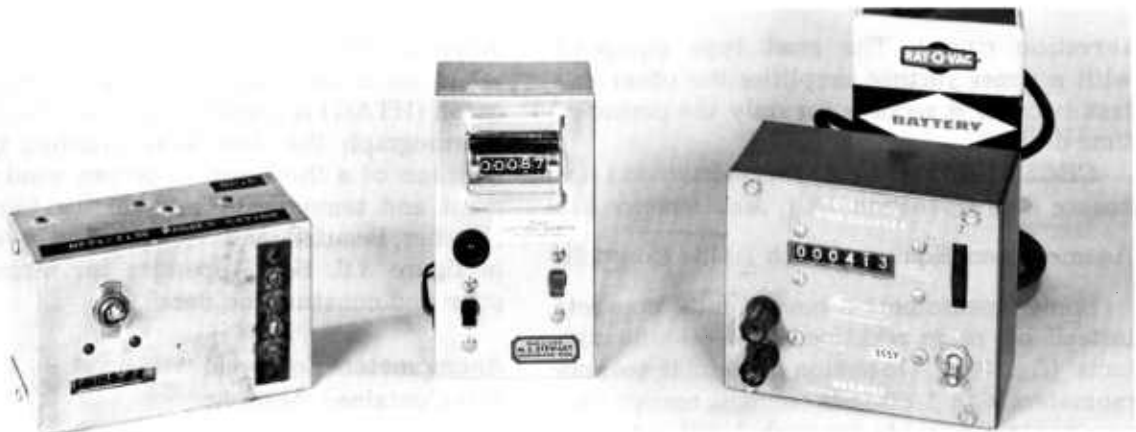
Figure 3.3. — Mechanical counters in use at fire-weather stations: Left and center, Nonreset types; right, reset type.
