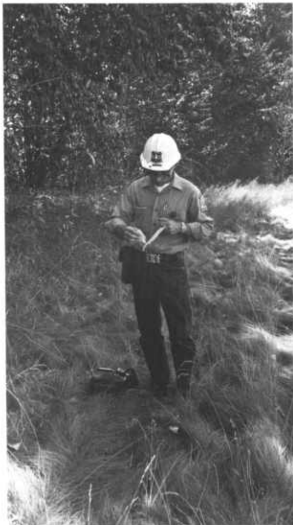
Figure 11.7. — Stand in shade. Wet the sling psychrometer wick prior to whirling.
