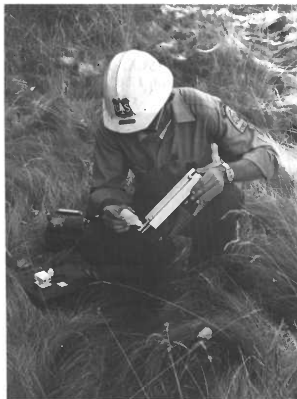
Figure 11.4. — Carefully wet wick. Avoid getting water on dry bulb.
