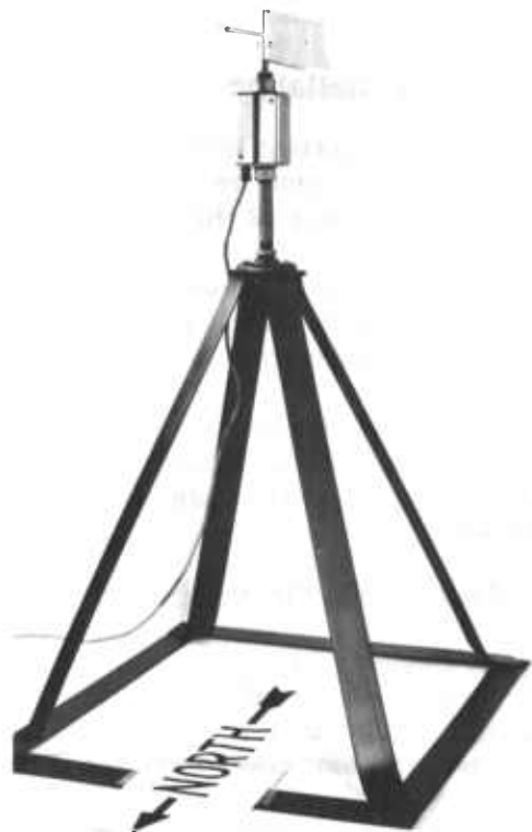
Figure 8.13. — Wind vane with scribe mark to assist in true north orientation.
