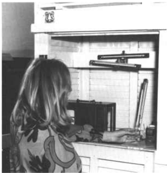
Figure 11.2. — Thoroughly wet the wick of electric fan psychrometer prior to taking measurements.
