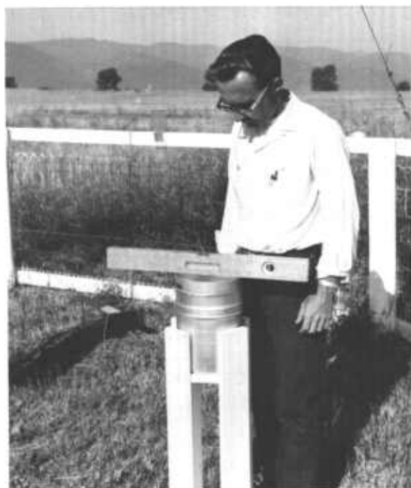
Figure 22.1. — Checking level on standard rain gage.
