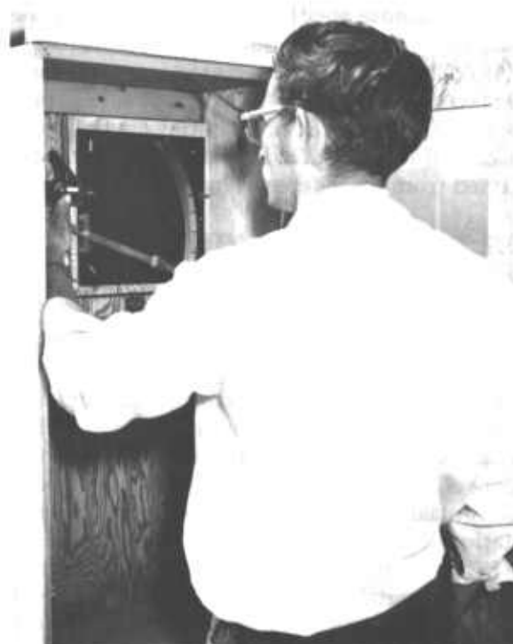
Figure 8.18. — Appalachian scale installed in an Appalachian shelter. Both the shelter and the scale should be level and plumb.
