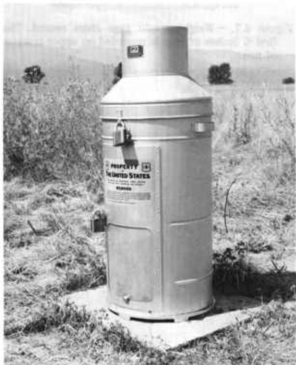
Figure 4.6. — Fergusson type weighing rain gage: Left , Assembled gage; right , weighing and recording mechanisms.
