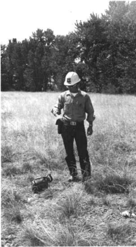
Figure 11.9. — Whirl psychrometer in body shade if no other shade is available.
