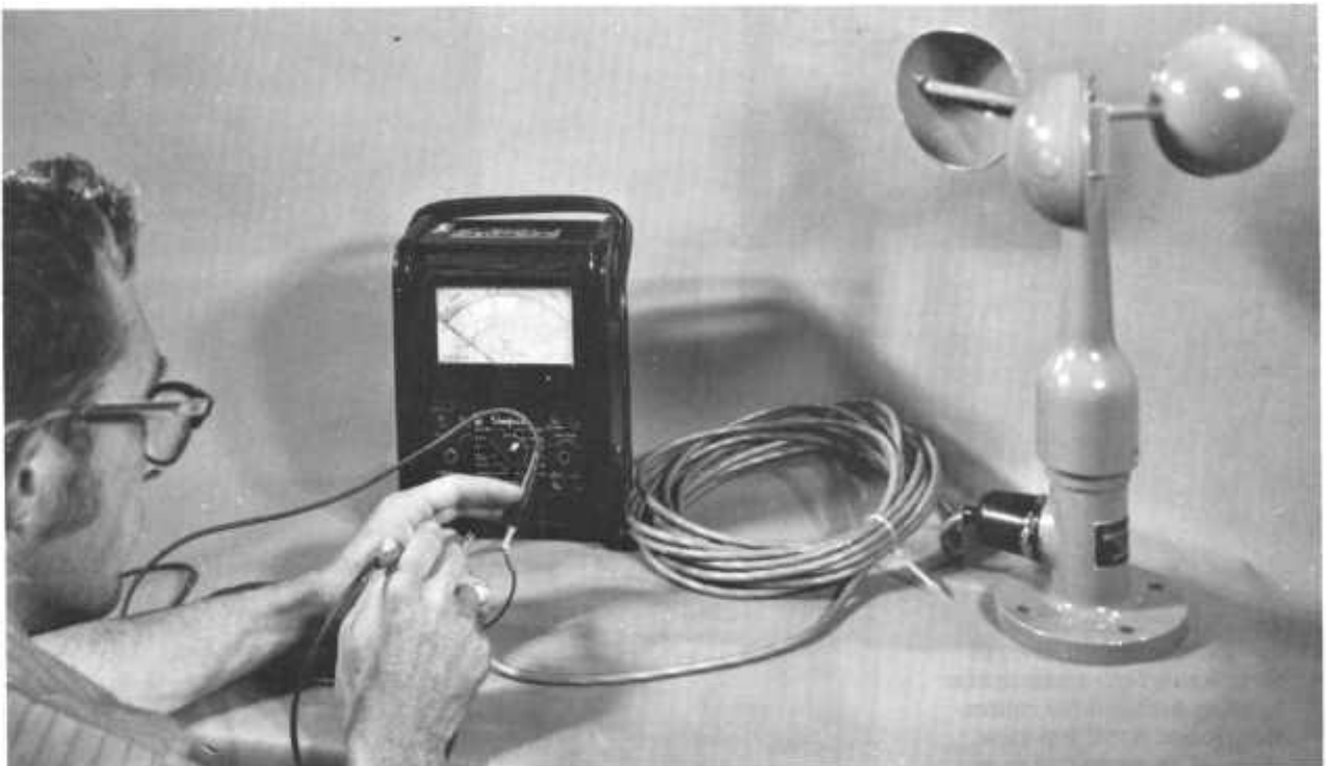
Figure 19.2. — Using a continuity tester to check an anemometer circuit.
