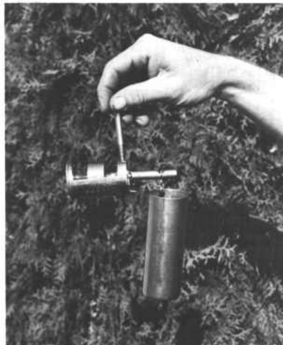
Figure 15.6. — Check calibration of scale by using cover as a 100-gram test weight.
