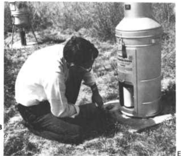
Figure 14.4. — Weighing rain gage operation: A , Remove collector; B , empty bucket; C , install fresh chart; D , wind clock; E , zero pen.
