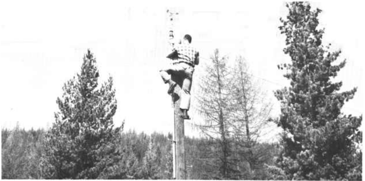
Figure 8.6. — This anemometer installation allows easy access to the anemometer and provides for periodic height adjustment. The wire on the right of the pole connects the anemometer to a wind counter located in the fire dispatcher's office.
