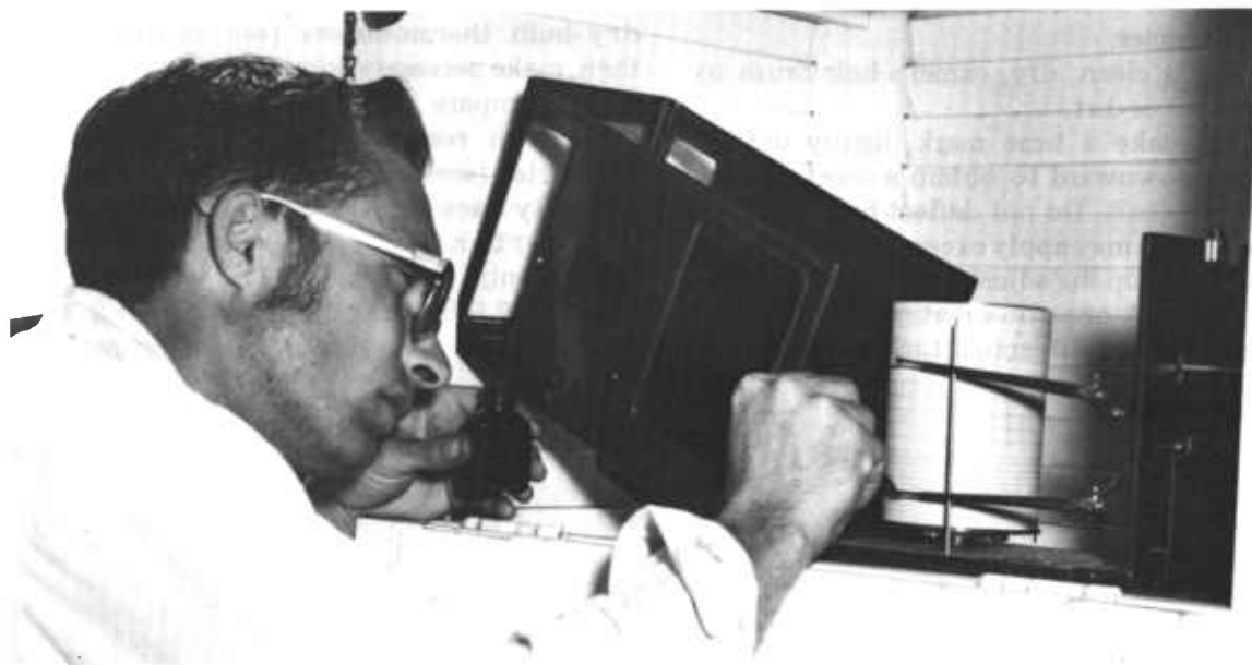
Figure 12.3. — Inking the pens of a hygrothermograph.
