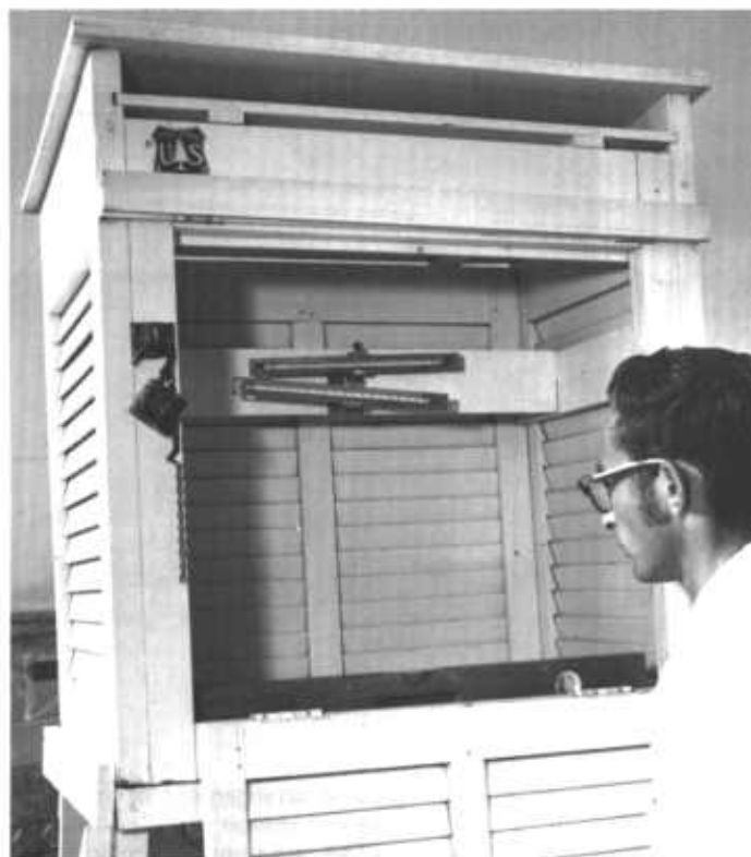
Figure 8.2. — Installing and leveling instrument shelter using mounting pins.
