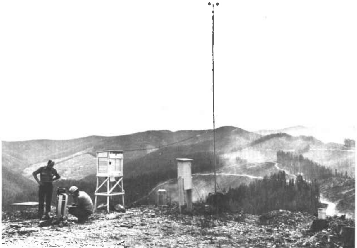
Figure 8.7. — This temporary anemometer installation was established to monitor weather for prescribed burning operations.
