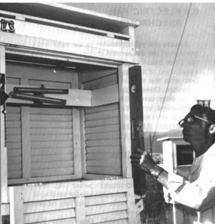
Figure 8.2. — Installing and leveling instrument shelter using mounting pins.
