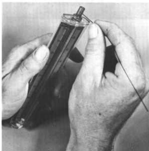
Figure 19.13. — Top , Cleaning, drying, and removing static from inner tube; bottom , cleaning top stem pinhole.
