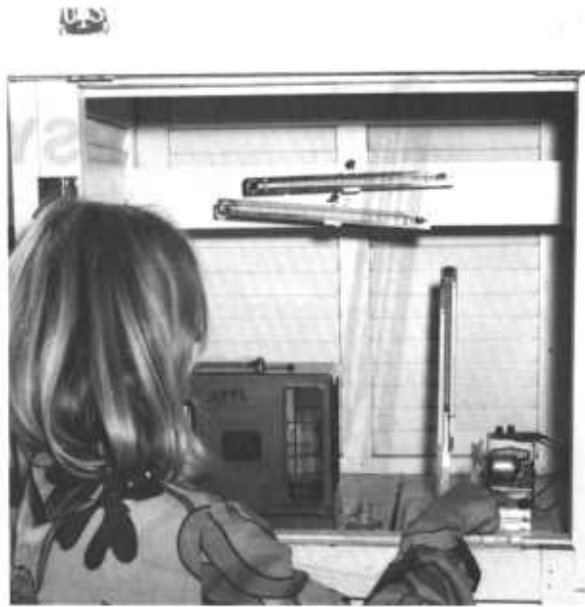
Figure 11.3. — Do not wet the wick during ventilation of the thermometers.
