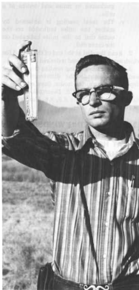
Figure 13.4. — Face wind and cover top stem with finger to measure winds in excess of 10 m.p.h.
