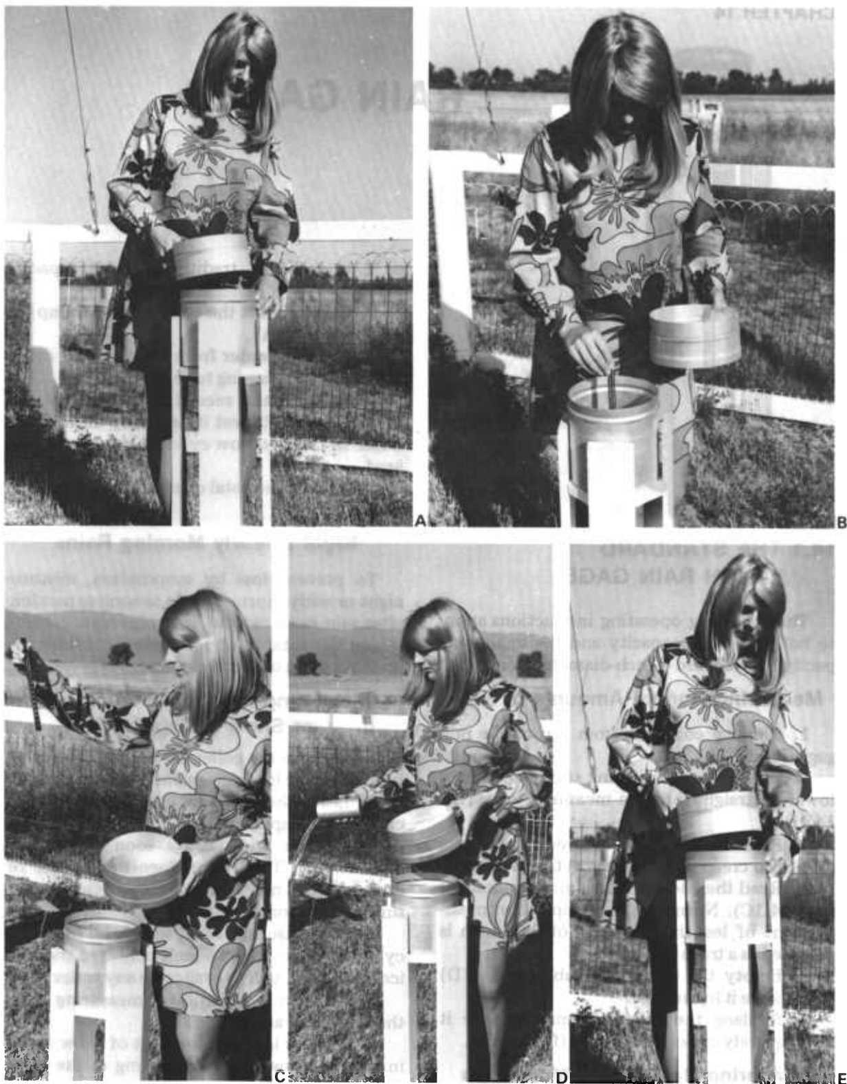
Figure 14.1. — Measuring normal amounts of rain with FS rain gage: A, Remove collector; B, dip measuring stick into inner tube; C, read stick; D, empty tube; E, replace collector.
