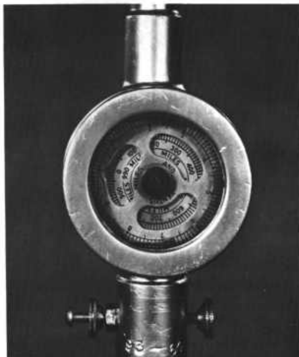
Figure 3.7. — Dial on this anemometer accumulates total wind movement past anemometer cups.
