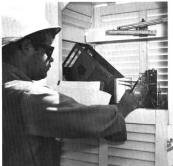
Figure 3.6. — A hygrothermoaerograph (HTAG). Uppermost pen arm has been installed to record wind movement.
