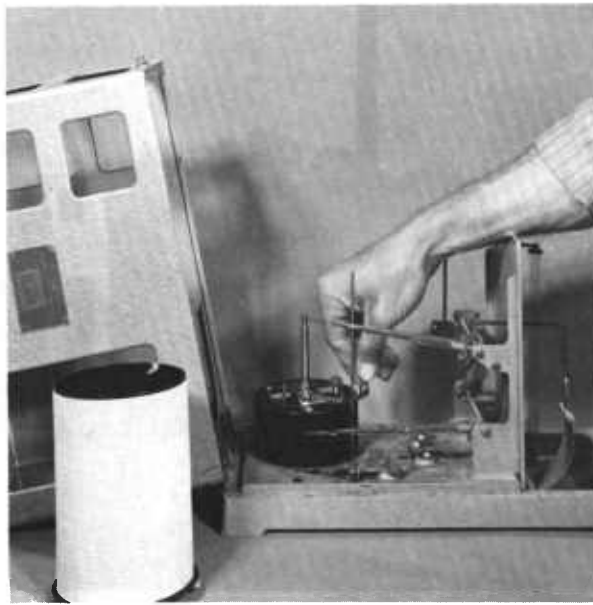
Figure 12.1. — Winding clock on hygrothermograph: Left , Clock in drum type; right , clock on base type.
