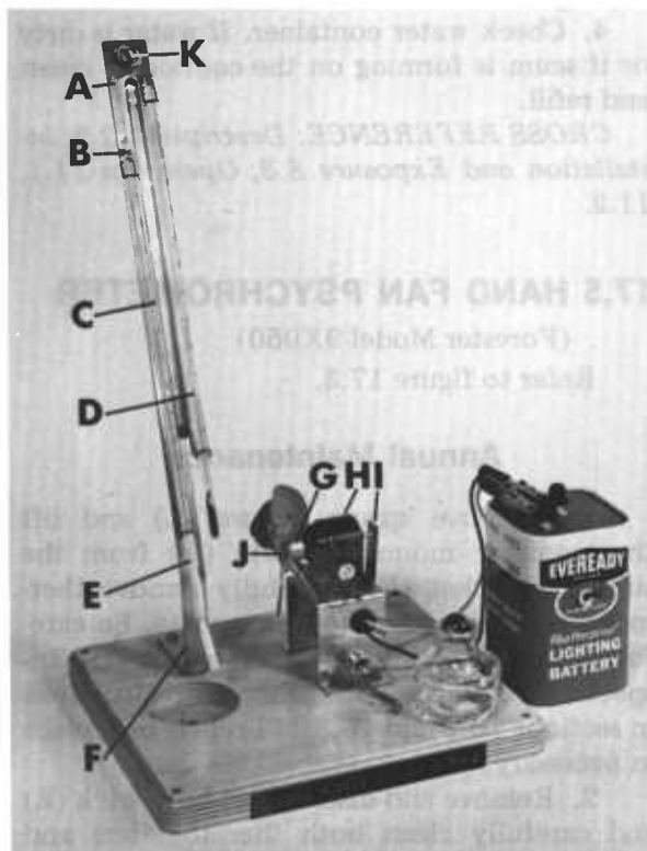
Figure 17.2. — Forester 9X060 electric fan psychrometer (left) and Forest Service electric fan psychrometer (right): A, Thermometer mounting plate; B, thermometer retaining screws and clip; C, wet-bulb thermometer; D, dry-bulb thermometer; E, wet-bulb wick; F, support bracket; G, fan and shaft; H, motor; I, thrust plate; J, fan bushing; K, spacer screw.
