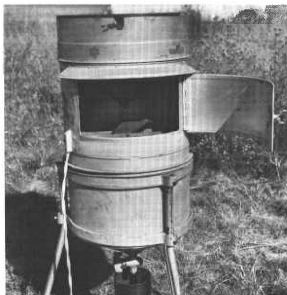
Figure 4.10. — Tipping bucket is visible inside the inspection door.
