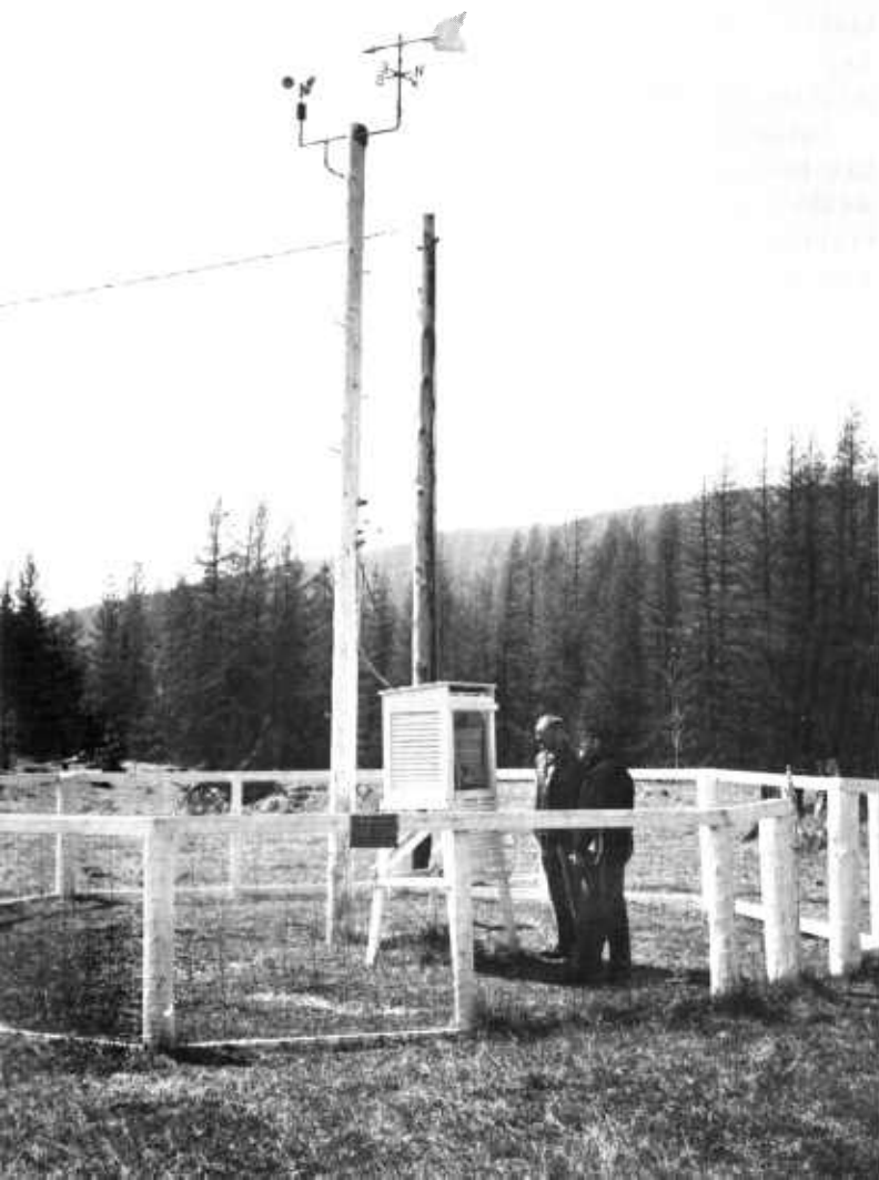
Figure 3.1. — Anemometer (windspeed) and wind vane (wind direction) exposed at 20-foot standard height at a fire-weather station.
