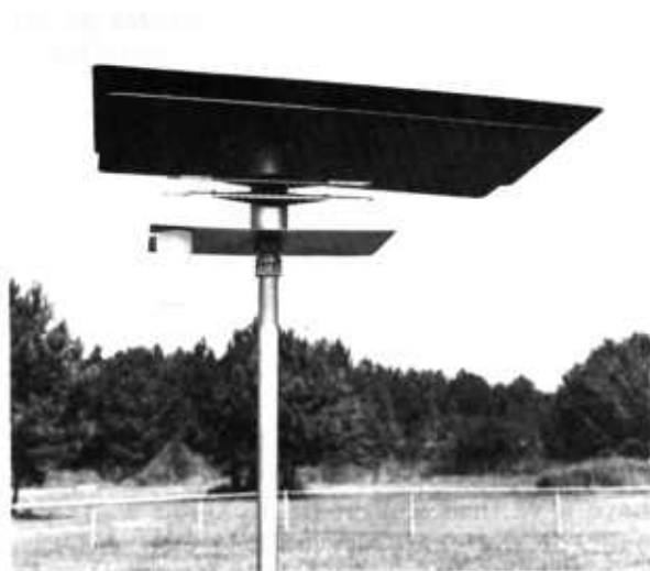
Figure 2.6. — The mortarboard psychrometer. This instrument is widely used in the Eastern United States.
