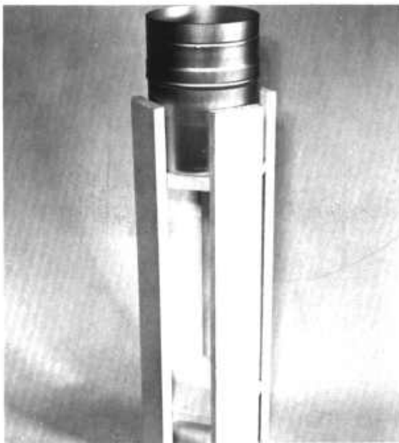
Figure 4.3. — Low capacity USDA Forest Service rain gage was designed for use in areas of low summer rainfall.
