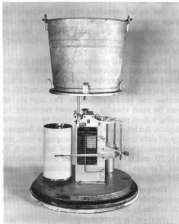
Figure 4.6. — Fergusson type weighing rain gage: Left , Assembled gage; right , weighing and recording mechanisms.
