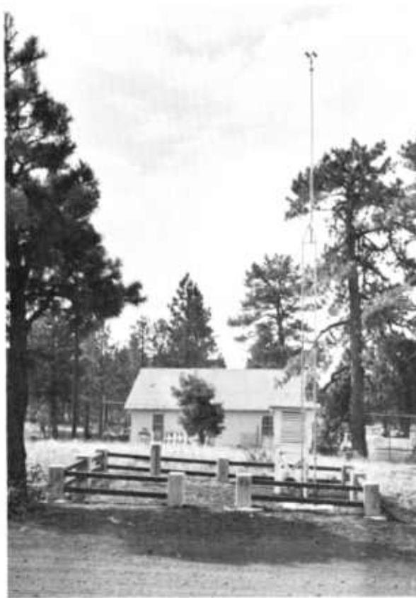
Figure 8.5. — In these installations the anemometer height is adjusted upwards because of nearby trees.
