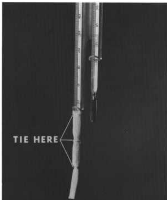
Figure 17.1. — A properly installed psychrometer wick.
