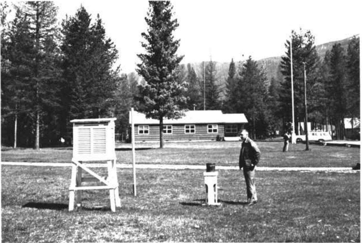
Figure 4.2. — Large capacity National Weather Service standard 8-inch rain gage.
