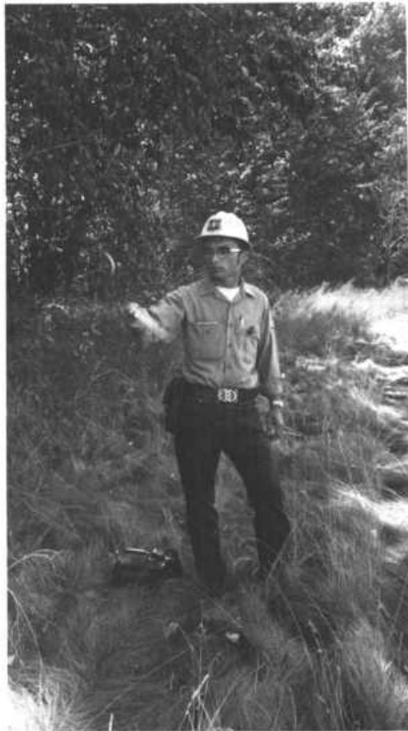
Figure 11.8. — Whirl sling psychrometer at full arm's length.
