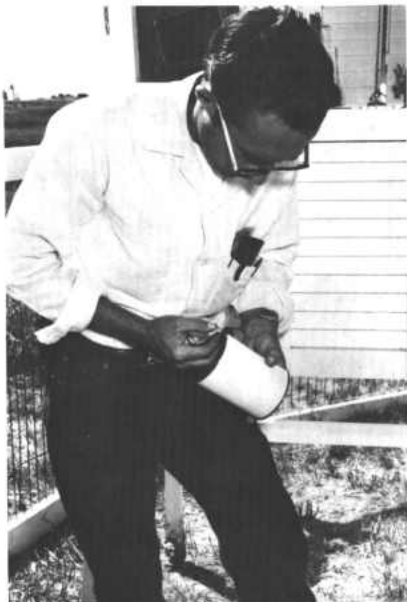
Figure 12.2. — To avoid losing part of the hygrothermograph record, install tapered charts on non-slotted cylinders.
