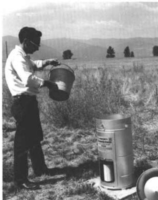
Figure 14.4. — Weighing rain gage operation: A , Remove collector; B , empty bucket; C , install fresh chart; D , wind clock; E , zero pen.
