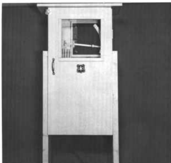
Figure 5.2. — Appalachian fuel moisture scale mounted in Appalachian scale shelter.
