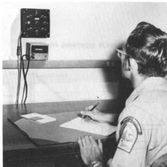
Figure 8.10. — The wind counter and wind direction indicator are often installed in the fire dispatcher's office.
