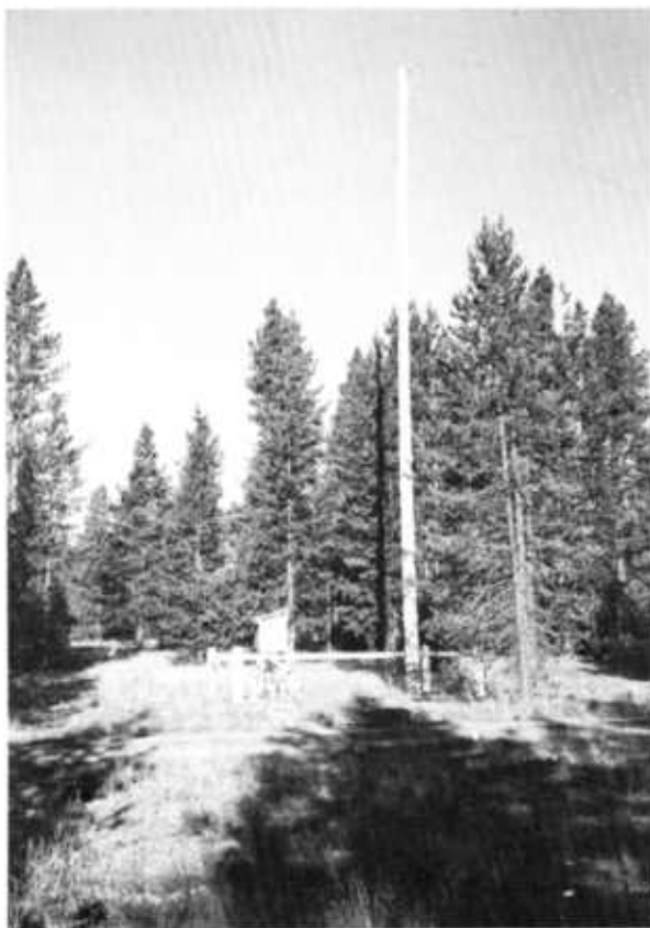
Figure 8.5. — In these installations the anemometer height is adjusted upwards because of nearby trees.
