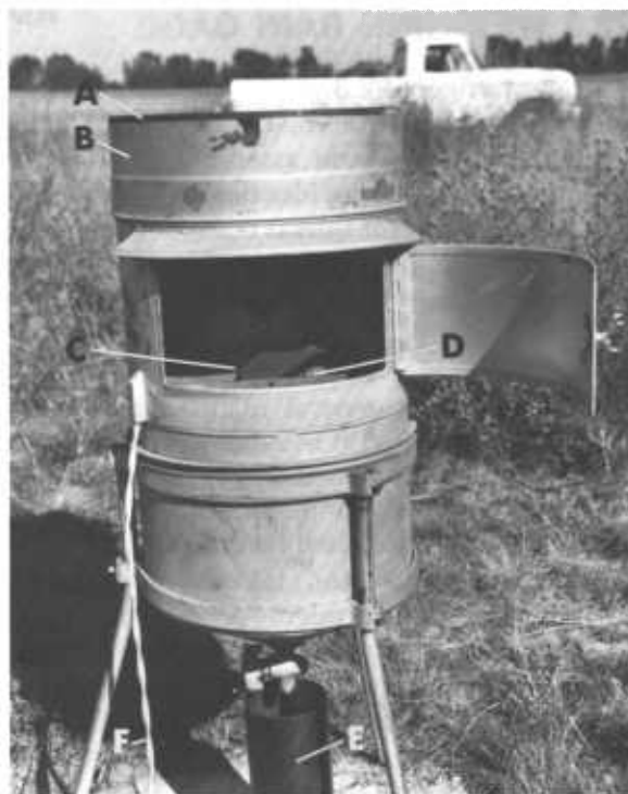
Figure 22.2. — Tipping bucket rain gage: A, Collector rim or knife edge; B, collector; C, tipping bucket; D, calibration stop screw; E, water storage container; F, cable to recorder.
