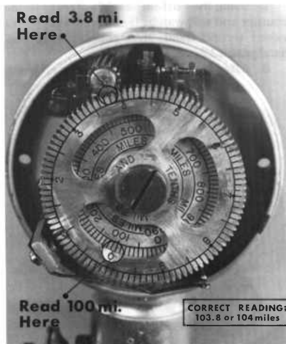
Figure 13.2. — Detailed view of anemometer dial. Dial indicates 104 miles of accumulated air movement past the anemometer cups.
