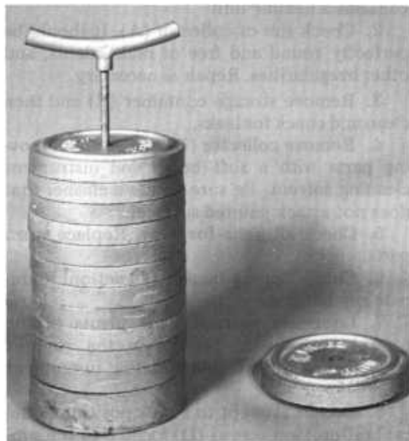
Figure 22.4. — Calibration weights for recording rain gages.
