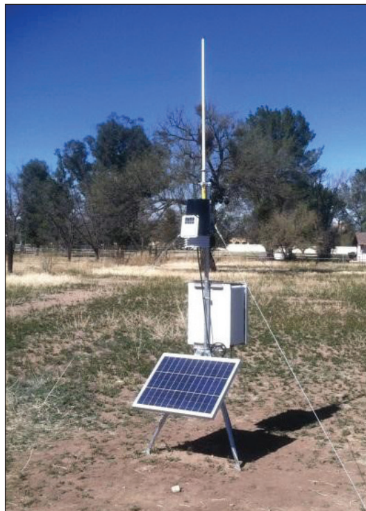
Figure 2-1. The Davis real-time weather station at Tumacácori NHP. Data are available through www.climateanalyzer.org .
