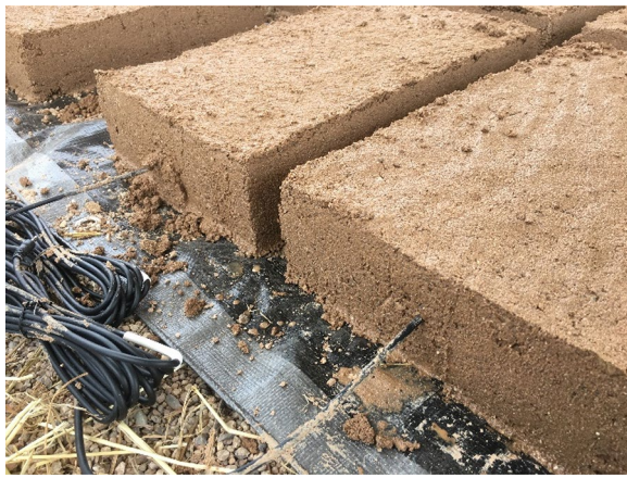
Fig. 1 Adobe blocks drying, showing placement of sensors
