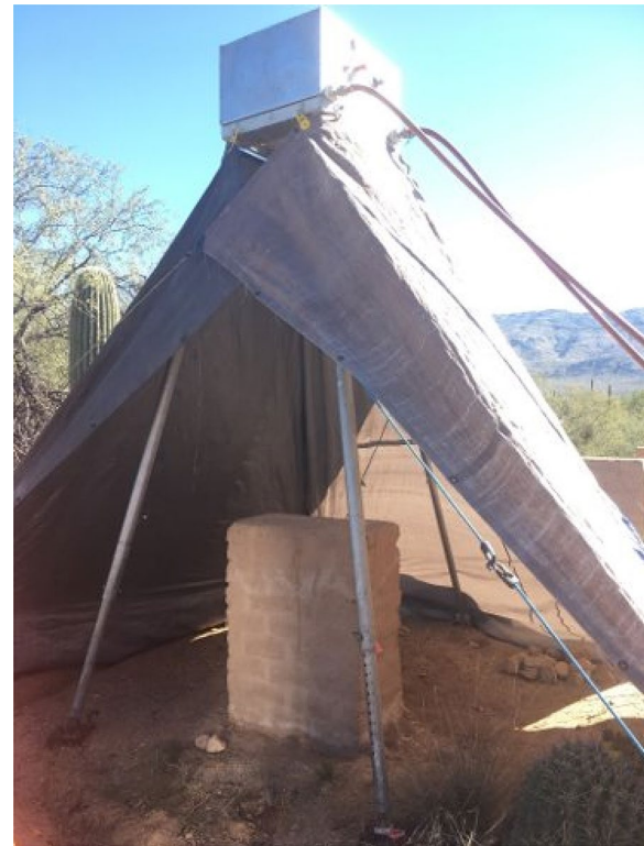
Fig. 3 Adobe test wall with rainfall simulator and windscreen set up
