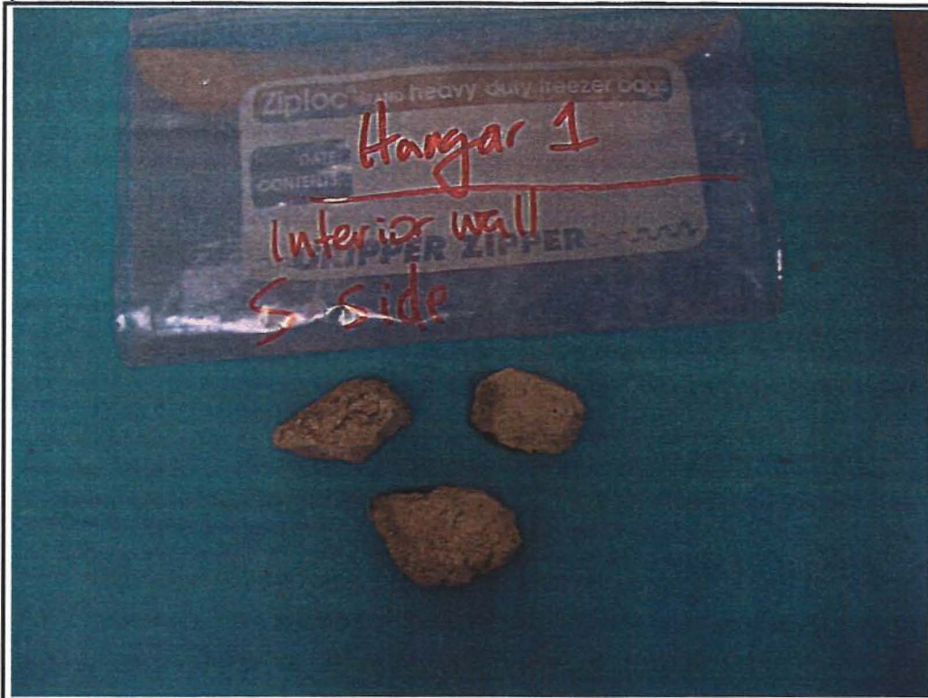
Photo 13. Hangar No. 1, Interior South Side— Mortar taken from brick
