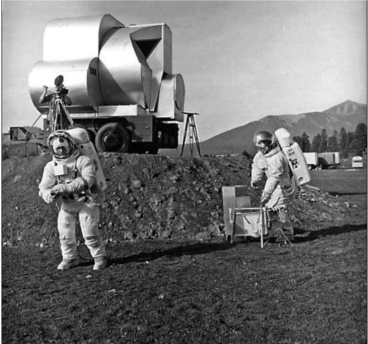
Fig. 70. Suited subjects Tim Hait and David Schleicher test tools at Cinder Lake Crater Field One with a mock Lunar Module in the background. The ramp was necessary to simulate the
