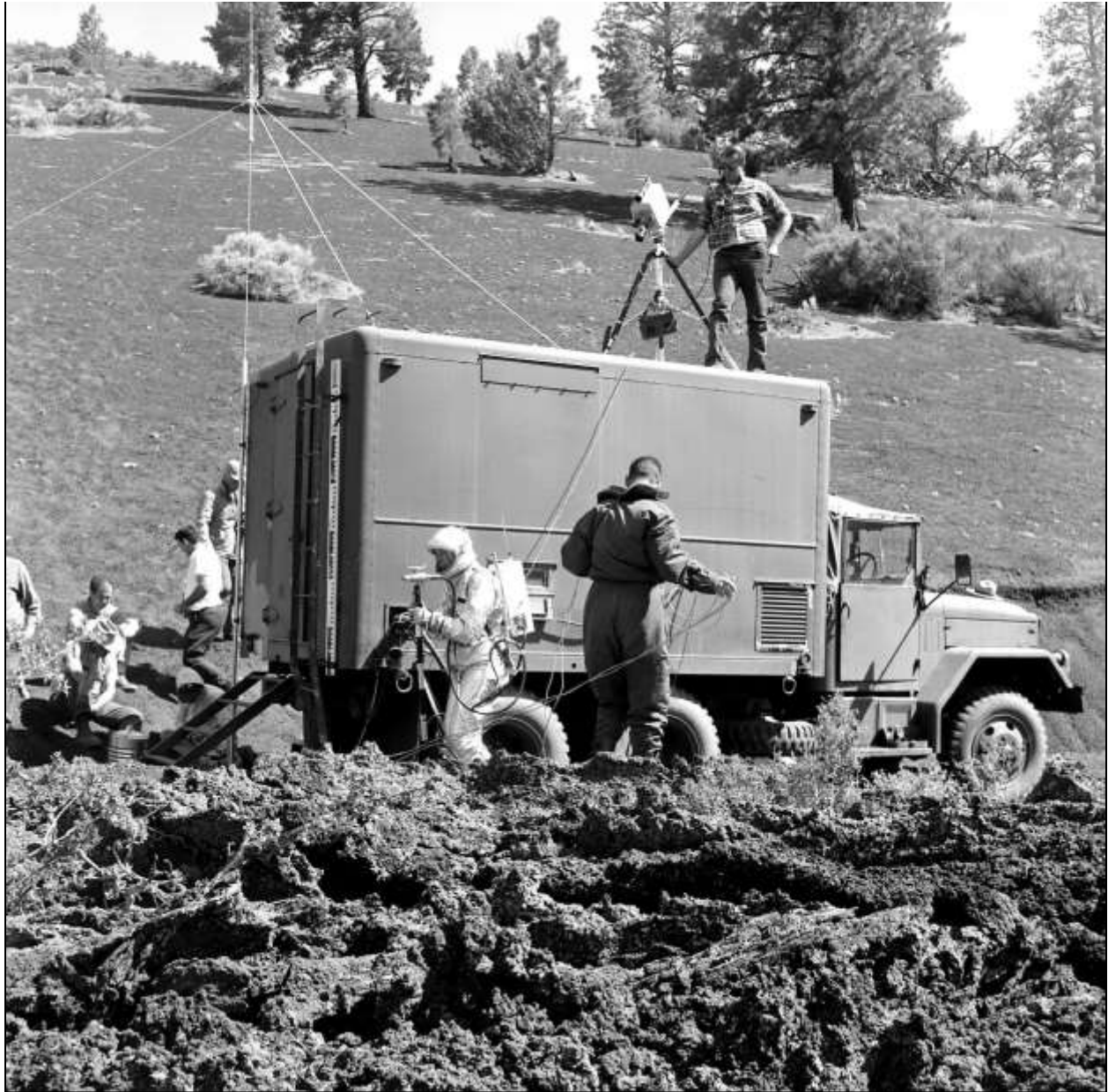
Fig. 77. USGS Branch of Astrogeology conducts their first spacesuit test on the access road within the North Bonito Lava Flow Test Area in June 15-20, 1964. The suited test subject (either Gene Shoemaker, G. Phillippi, or J. Harbour) is visible in front of the support van holding a prototype lunar staff for taking pictures. The general characteristics of the site are evident here including the sharp distinction between the cinder hill and a'a lava flow. (Photo by Paul Long. Image from Schaber, open-file report, 2005).
