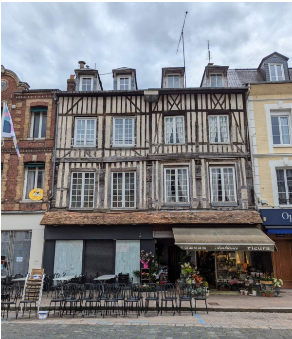
Figure 24. 17th century, close-stud pan-de-bois buildings in Pont-Audemer, Normandy, France, showing a typical configuration for urban buildings with multiple stories and shared party walls. (Source: Lurita McIntosh Blank, 2024)
