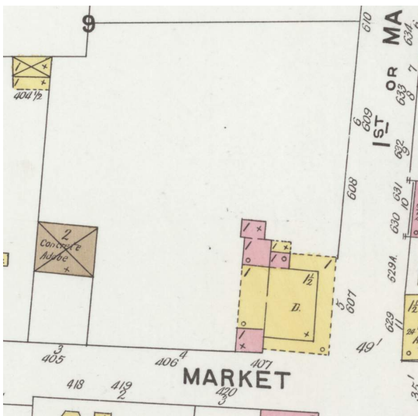
Figure 4. 1901 Sanborn Fire Insurance Map, showing the Vallé House parcel. Yellow indicates frame lumber construction, and pink indicates brick construction. The stable (designated by the X) is now shown as a two-story "Concrete Adobe" structure of a similar footprint. (Source: Library of Congress)
