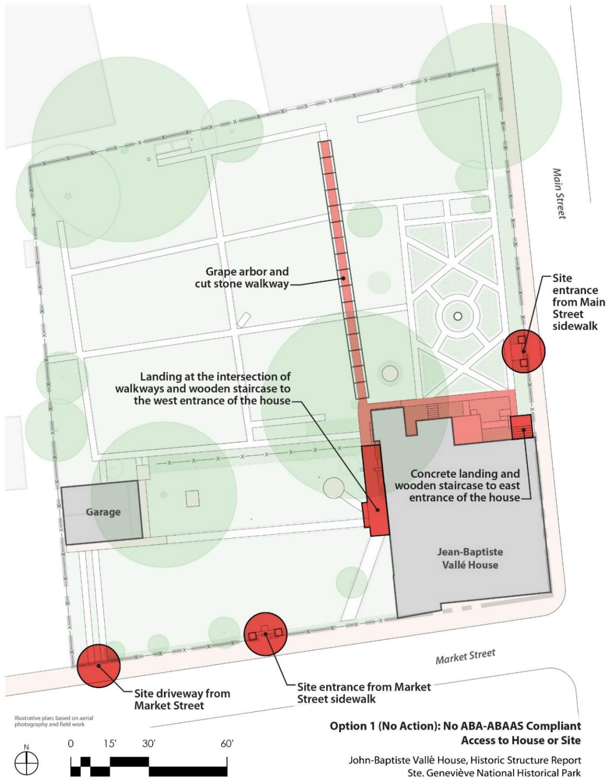
Figure 1. Treatment Option 1: Existing Conditions: No ABAAS Compliant Access to the Jean Baptiste Vallé House and Landscape. (Source: LSHLA)
