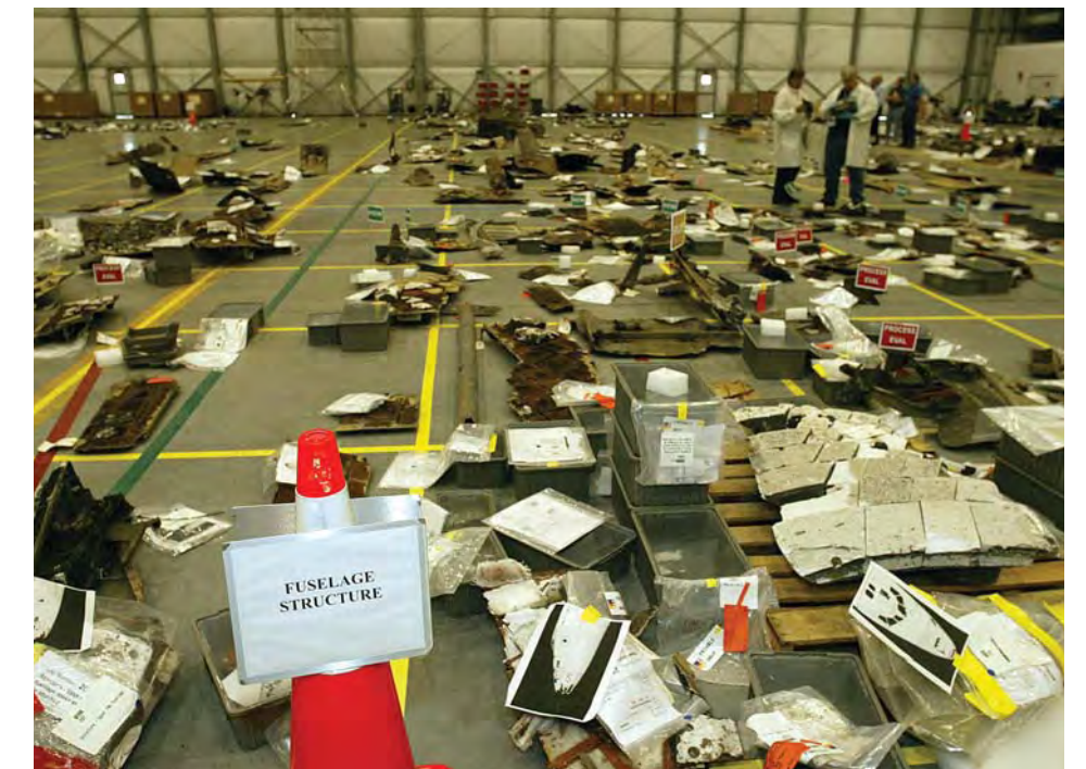
Looking down the line of identified main fuselage debris located on the grid system in the Columbia debris hangar.
