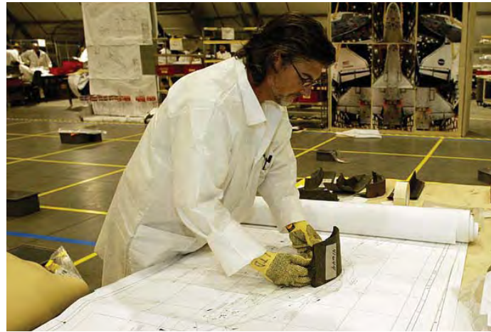
A reconstruction team member uses 1:1 engineering drawings as a tool in the process of identifying recovered debris material.
