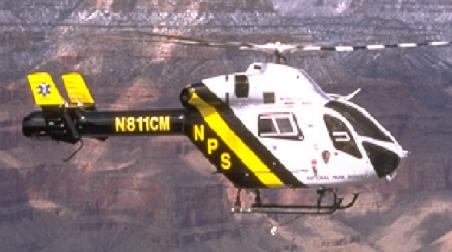
Grand Canyon National Park is reducing noise from NPS aviation use by flying an MD-900 Explorer NOTAR (No TAil Rotor) helicopter for park operations. In addition, area tour operators are joining NPS efforts to implement quiet technology and restore natural quiet.
