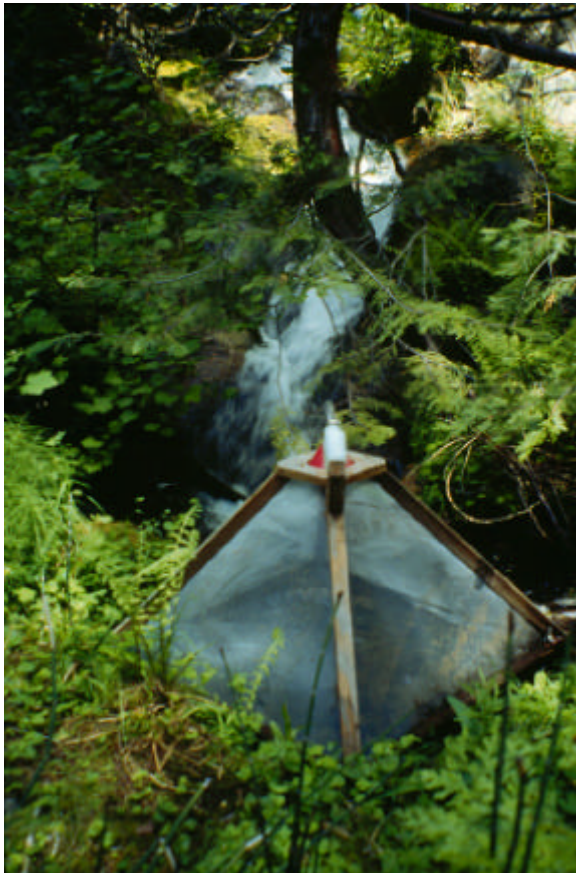
Figure 32. Pyramidal trap used to capture adult macro-invertebrates (photo by C. Moore).
