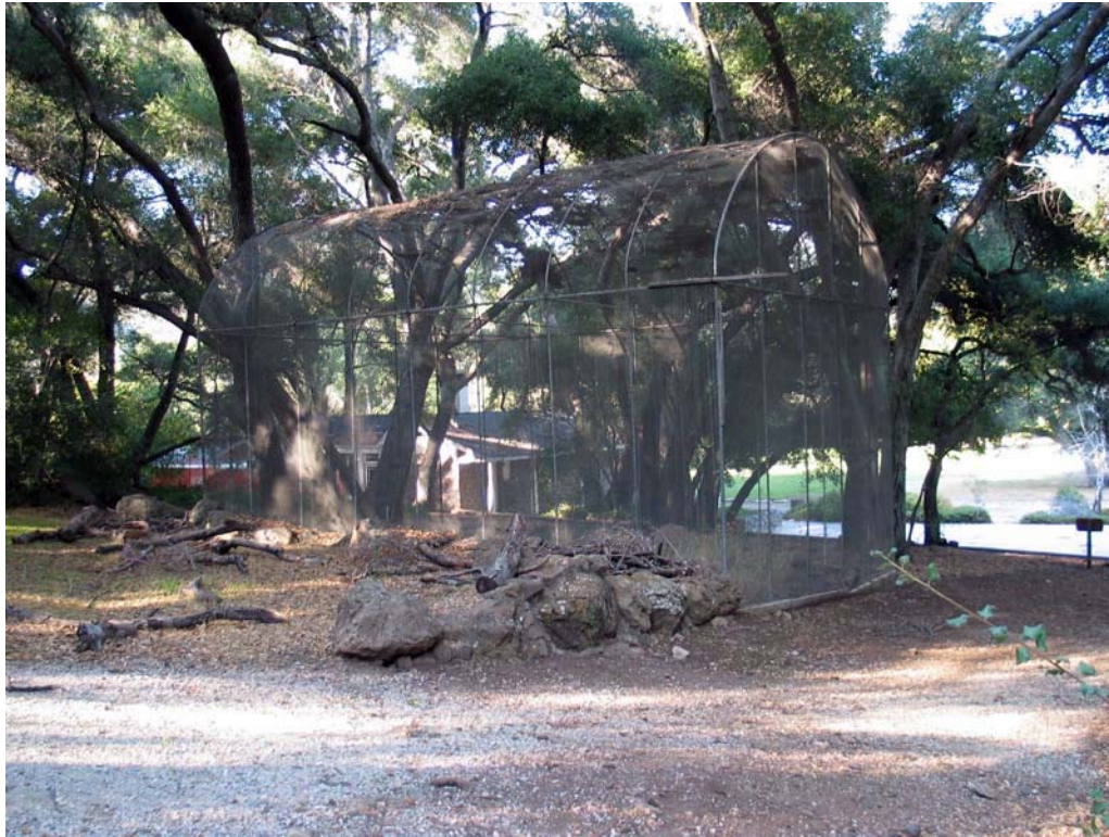
Buildings and Structures Photo #4. The aviary, constructed of a galvanized pipe frame and metal mesh, was part of Harry Miller's ranch. (PWRO 2005)
