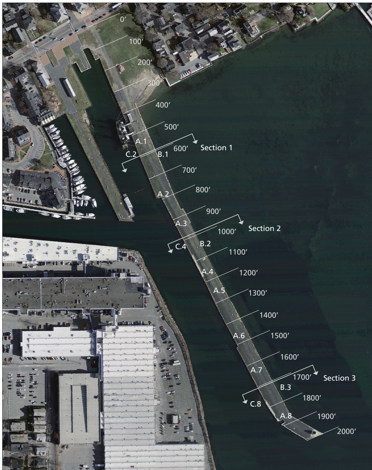
Figure A.09. Aerial photograph with overlay showing one hundred foot intervals along the length of Derby Wharf. Photographs at intervals are shown in Figure A.10. Three sections indicated above are illustrated in Figures A.11, A.12, and A.13 (OCLP).
