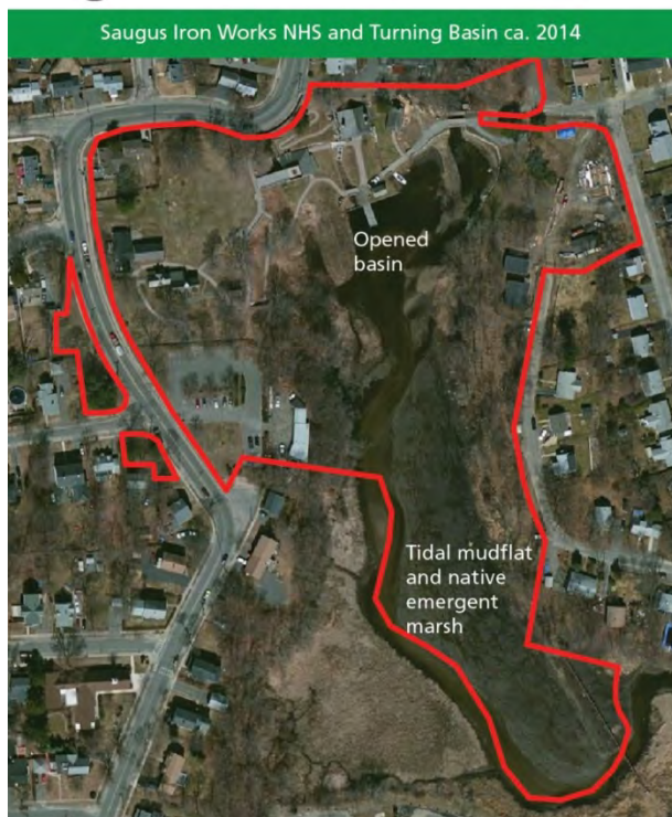
Figure 18. Turning Basin restoration. Pre-restoration conditions (upper image) contrast with post-restoration conditions (lower image). Restoration efforts removed invasive aquatic species and dredged sediments to restore native species and historic settings. The loading dock, once used to transport goods to and from river barges now connects to the Saugus River channel. Graphic by Trista L. Thornberry-Ehrlich (Colorado State University) modeled after figure 4 from James-Pirri et al. (2011) and using ESRI World Imagery basemap.
