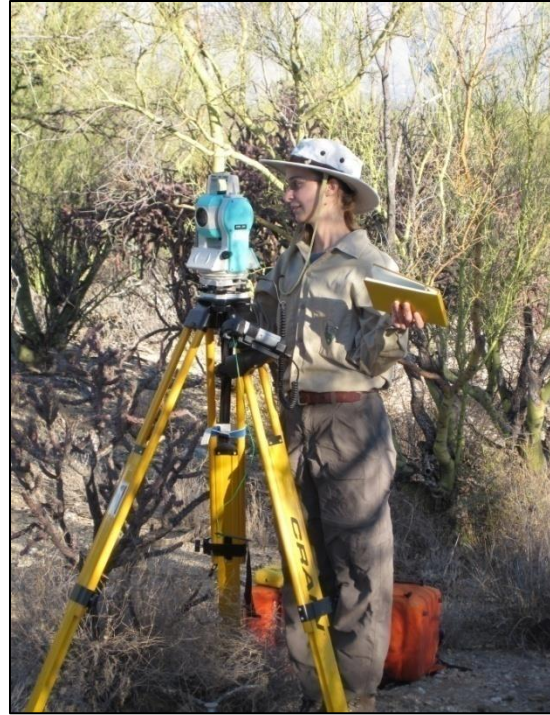
Figure 4. Operation of the Nikon DTM-330 Total Station Transit and prism pole by Saguaro National Park employees Chris Hannum (l) and Kris Ratzlaff (r).
