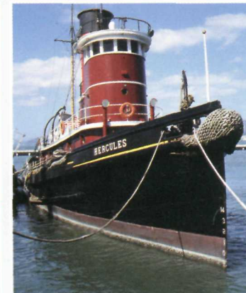
Hercules : steam-powered tug boat; 139 feet. Built 1907 Camden, N.J.
