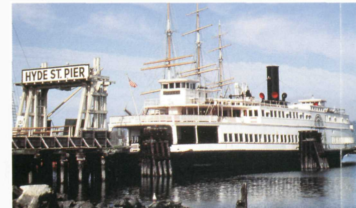
Eureka : side-wheel ferry; 299.5 feet. Originally built 1890 as Ukiah , Tiburon, Cal. Refitted 1922 as Eureka .
