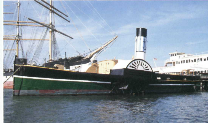
Eppleton Hall : steel tug boat; 100.5 feet. Built 1914 South Shields, England.
