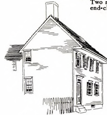
Gable roof and cornice overhang.
