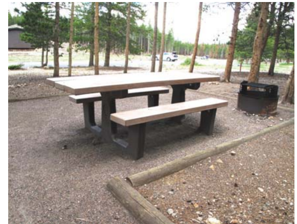
An accessible picnic table allows for inclusion of all visitors; a visitor using a wheelchair can comfortably fit at the end of the table. Also, the integral concrete color requires less maintenance-no painting.
