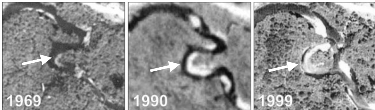
Figure 3. Three time periods of the same river reach showing it inundated by a beaver pond in 1969, active river bars in 1990, and abandoned by channel avulsion in 1999.
