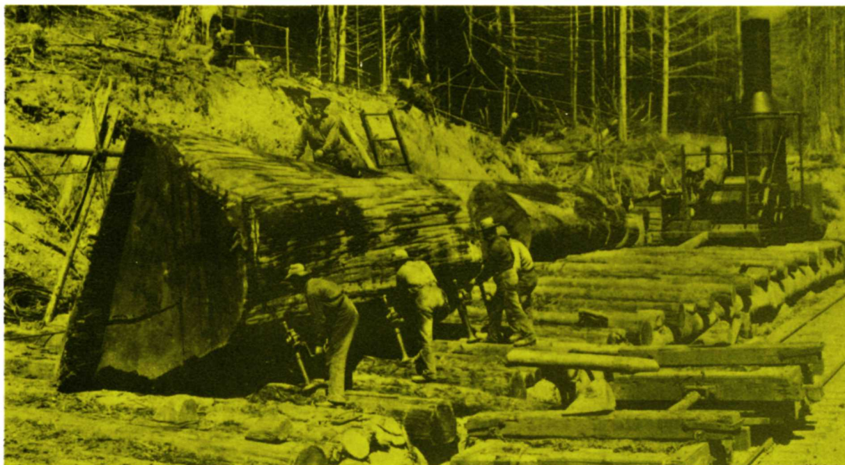
Jacking over a log preparatory to splitting it with dynamite.
