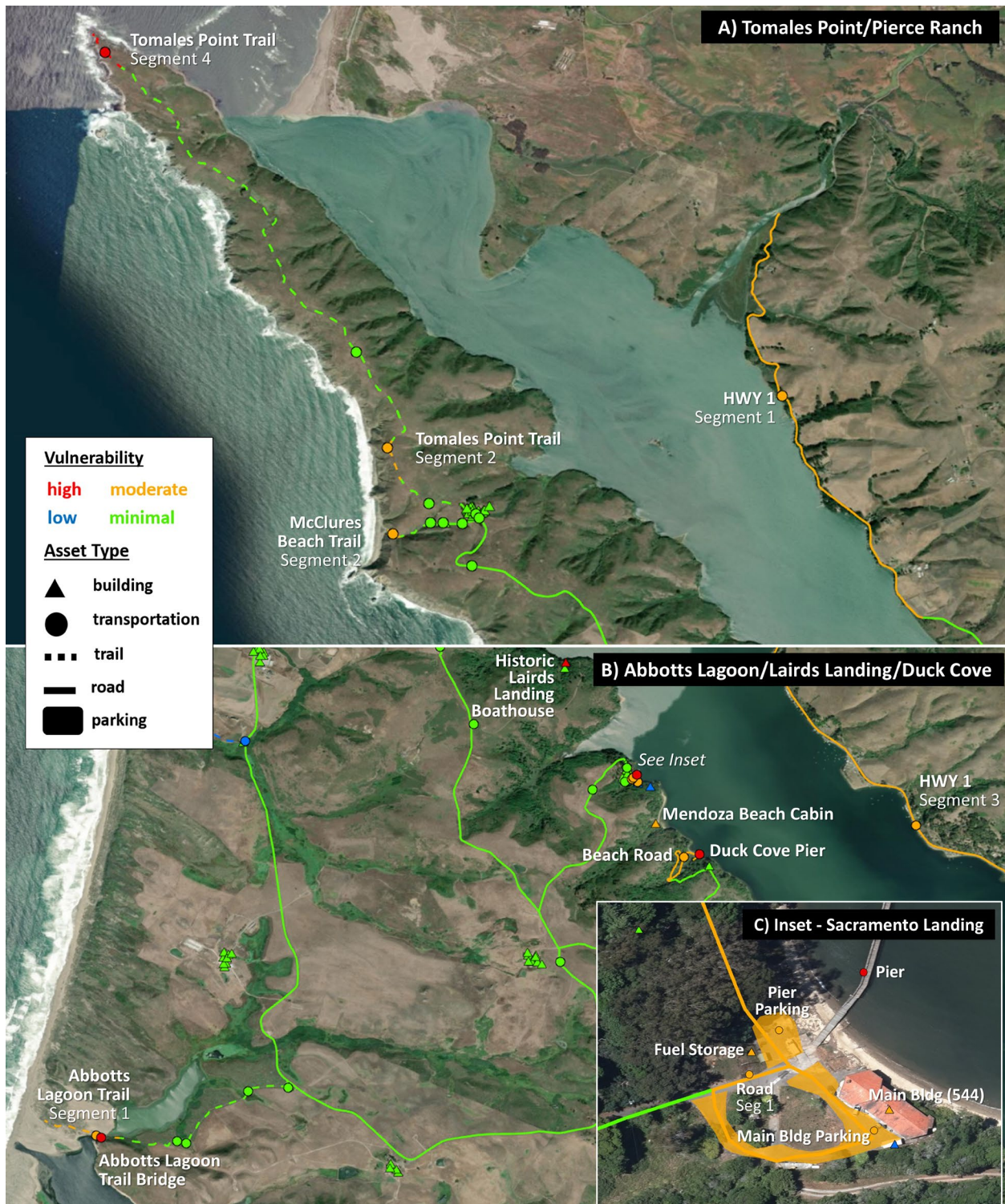
Figure 7. PORE vulnerability results summary for the A) Tamales Point/Pierce Ranch, B) Abbotts Lagoon/Lairds Landing/Duck Cove, and C) Inset – Sacramento Landing areas. Only high and moderate vulnerability assets are labeled. Background is 2023 ESRI world imagery.
