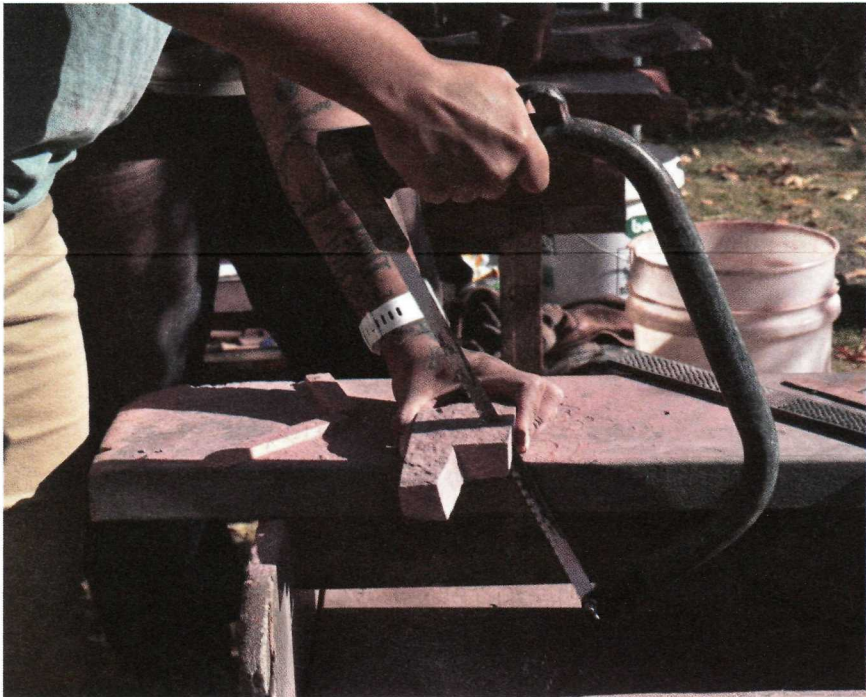
Above Left: Jessica Arkeketa carves out a pipe from a sheet of pipestone using just a hacksaw. Above Right: The stone is soft enough to then be shaped with a metal file, as Travis Erickson demonstrates.
