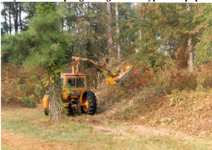
Brush mower with boom allows mowing without driving on earthworks. (Fort Wadsworth, 10/1994)
