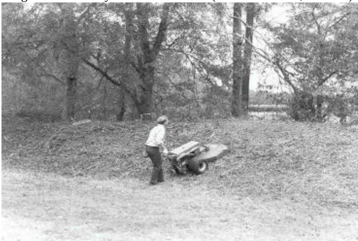
Walk-behind powered mowers mulch and cut remaining stubble down to ground level. (Fort Wadsworth, 10/1994)
