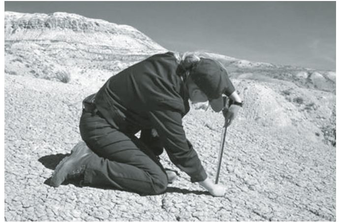
Figure 5. Installation, measurement, and documentation of erosion stakes at Fossil Butte National Monument in 2002. Such stakes provide quantitative local erosion rates and can be used in paleontological resource management prescriptions.
