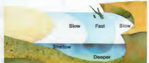
Cross Section of Typical River Bend
