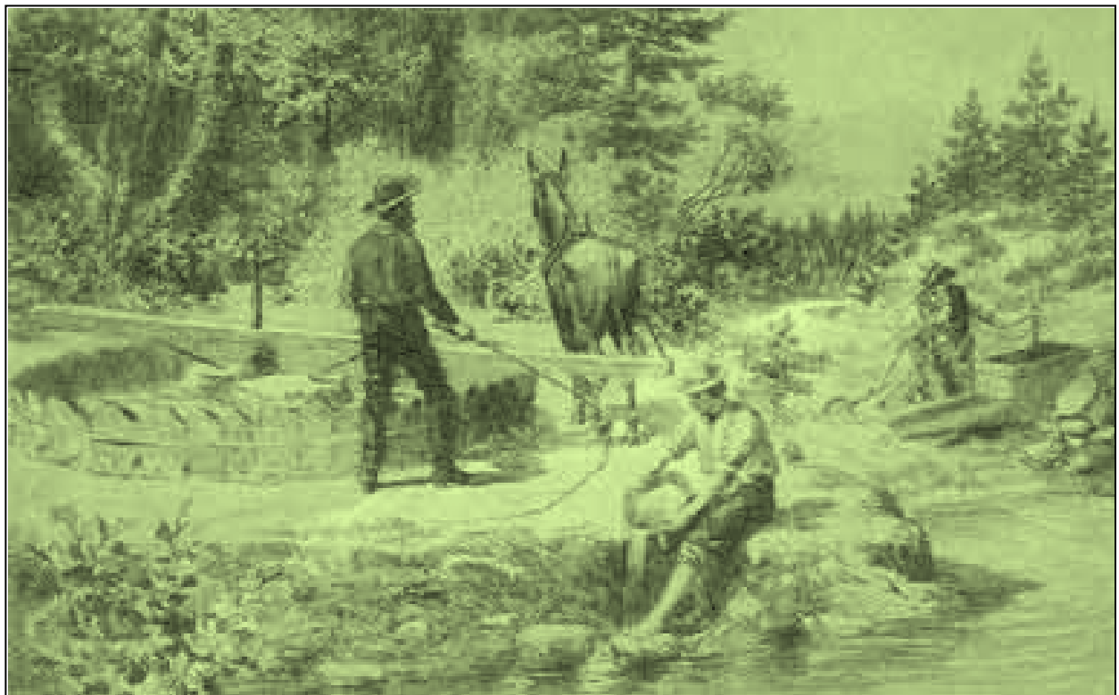
Figure 15. An arrastra. A draft mule or burro (or sometimes the miner himself) dragged a large boulder around and around large flat boulder netherstones set in a circle to pulverize and grind ore. Photo: Encyclopædia Britannica Online.
