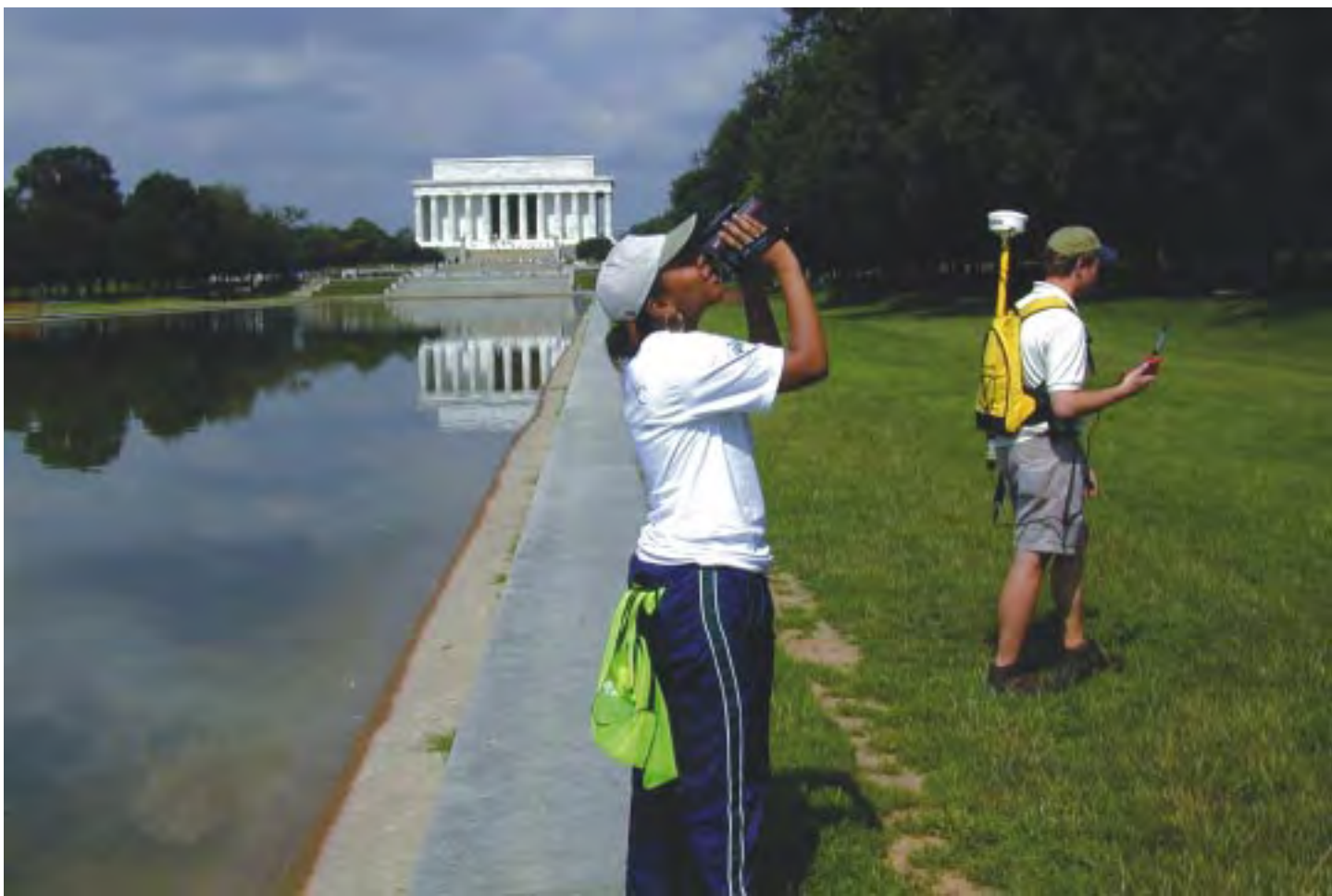
A forestry intern with the Casey Tree Foundation (left) uses a laser range finder to measure the height of the oldest and largest trees at the Reflecting Pool on the National Mall as an intern from the University of Maryland (right) provides GPS information for each tree measured.
