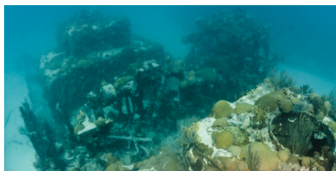
Figure 44: Mary Celestia 's engine room, looking forward from the aft boiler past the cranks of the double oscillating engines to the forward boiler.
