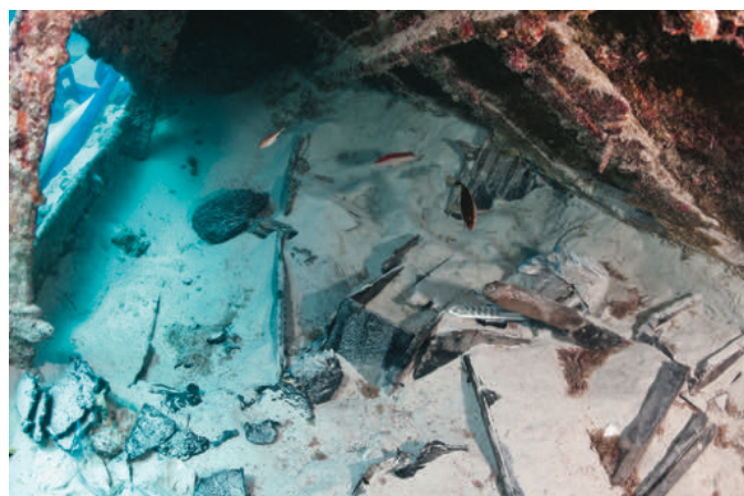
Figure 47a & b: Interior of the bow looking forward, showing the deck beams (left), the starboard hull with frames and the bilge keelson and bilge stringer (right) and the kingpost (center).
