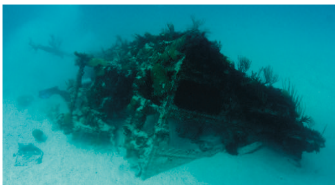
Figure 45: Mary Celestia 's bow with the exposed section of keel and keelson and the aft collision bulkhead. Also note the steam winch/windlass.
