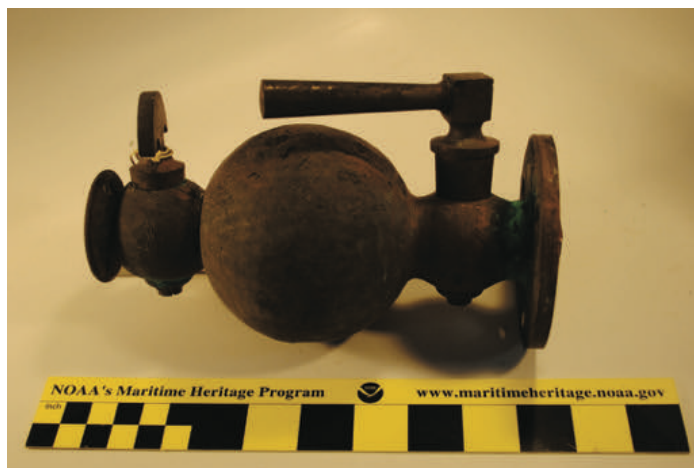
Figure 16: Brass globe valve recovered by Teddy Tucker in the collection of the National Museum of Bermuda, Acc. 260500, Cat. No. 808-4.
