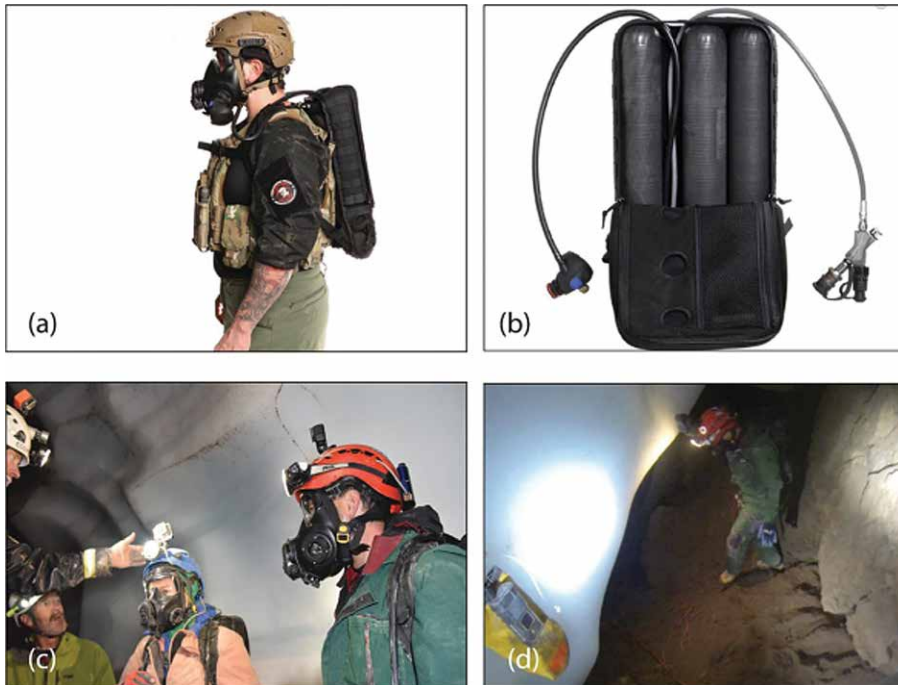
Figure 3. (a) Product image of Extreme Limited Access Breathing System (ELABS) Self Contained Breathing Apparatus (SCBA) showing thin confined space profile. (b) ELABS three carbon-fiber tank design, regulator, and air gauge/Rapid Intervention Team (RIT) quick fill connection. (c) Preparation to enter the "CO 2 Lake of Death" while wearing ELABS SCBA as life support equipment. (d) Descending into the "CO 2 Lake of Death" using ELABS SCBA as life support equipment.
