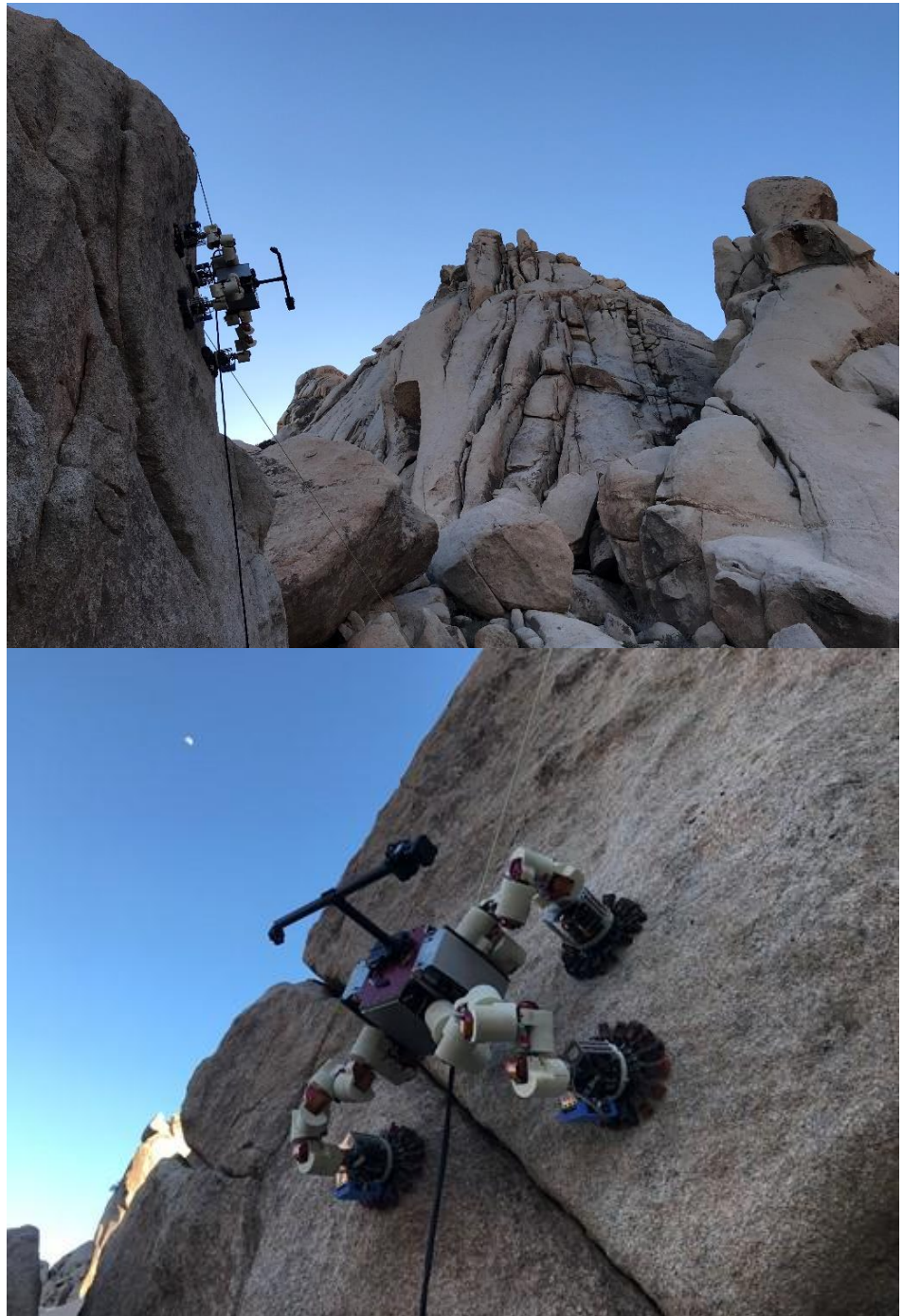
Figure 1. LEMUR scaling a nearly vertical granite outcrop at the Sweeney Granite Mountains Desert Research Center. Microspine gripper end effectors are attached to the chassis via seven degree-of-freedom limbs. A perception system consists of a camera and LIDAR mounted to a mast on the chassis. A safety line and a tethered power cable are also present above and below LEMUR.
