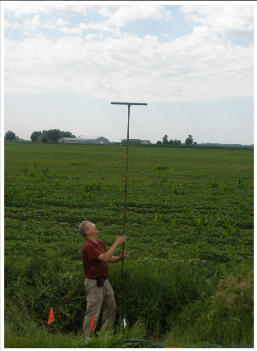
Tim Freed using soil auger to collect sediment samples. NPS Photo.
