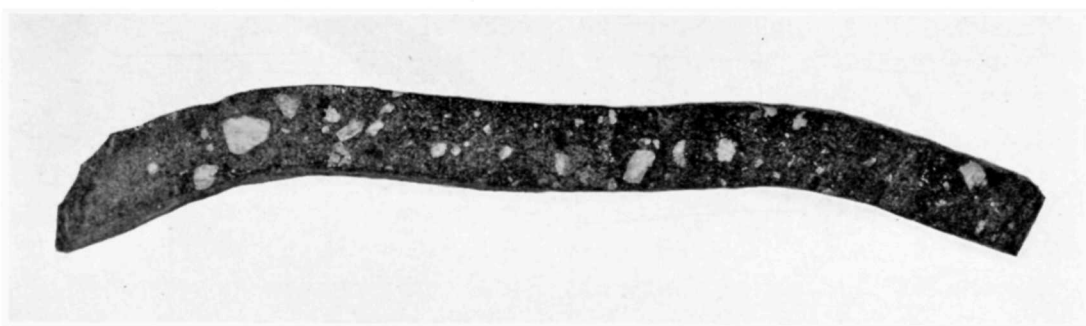
Fig. 28.—A prism of dense Lassen andesite, supported at two points and heated to 1040^\circ C. for 15 minutes. Note the sag at ends and center. Photo Snapp.
